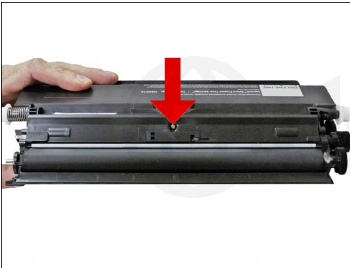
19. Re-install the developer roller cover and screw.
