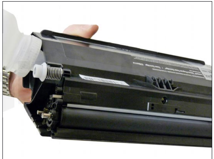
20. Fill the cartridge with the proper amount of toner for the Lexmark E260/360/460/X264/363/364 and install the fill plug.
