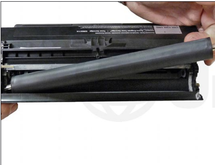
12. Remove the developer roller.
