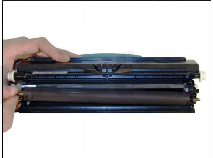
9. Wipe the developer roller with a clean lint free cloth, and re-install the developer roller. At this point we do not recommend that any chemicals be used to clean this roller. Install the keyed end of the roller to the gear side.
