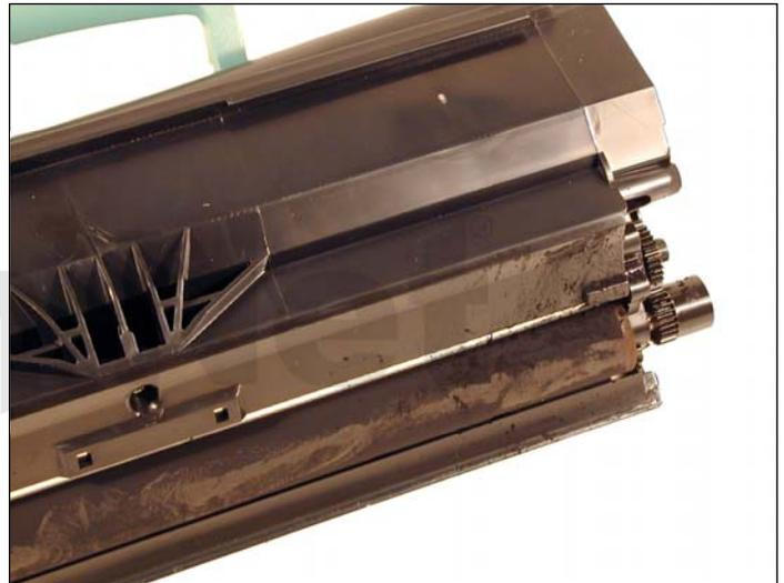
**Left image shows the cartridge with the new felt style cover. Right image shows a sample of the leakage found on just about every cartridge tested so far. None of the leakage showed on prints past the first or second pages, but it did show.**
