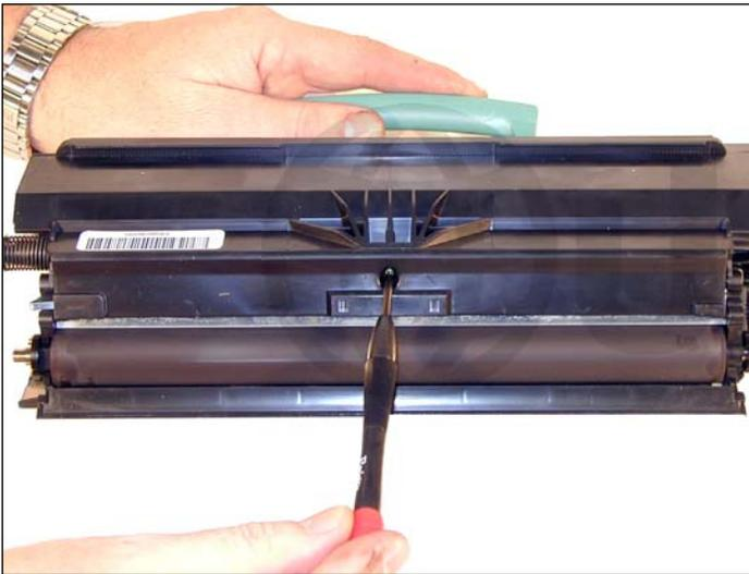
13. Re-install the developer roller cover and screw.
