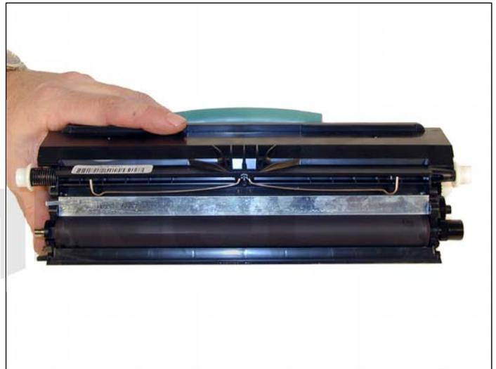
12. Install the doctor blade making sure it is positioned correctly and install the leaf spring.
