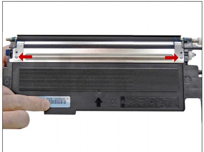
19. Carefully clean the cover/doctor blade and install it. Fit the individual doctor blade pressure plates on their proper sides and secure with the two screws.
