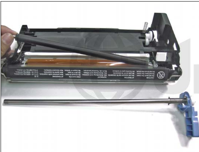
14. Remove the PCR and clean with a damp cloth.
