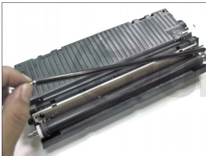
26. First, remove the toner charging roller by pulling it out sideways.
