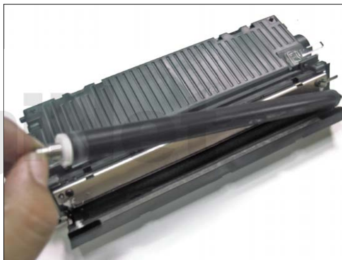
27. Remove the developer roller by pulling it sideways. Be careful not to lose the white bushings on each end as they can easily fall off.
