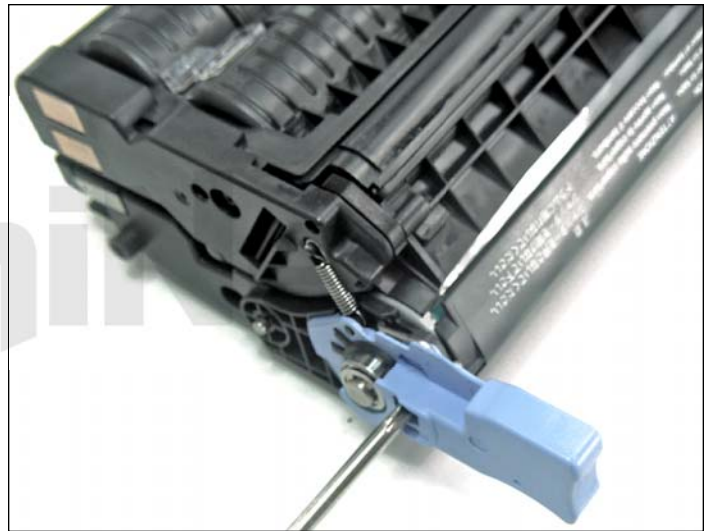
45. Install the blue cartridge handles.
