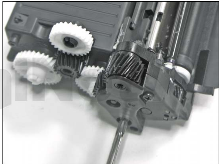
21. Remove the two screws on the gear side end plate.
