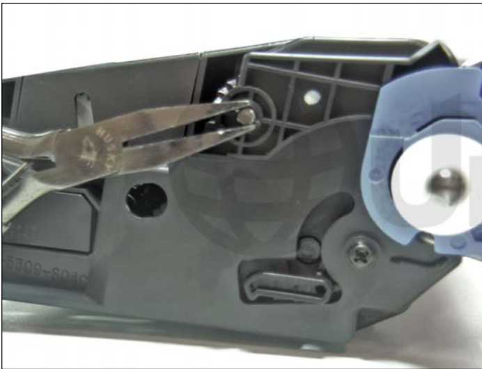
4. Grip the pin head with a pair of pliers.
