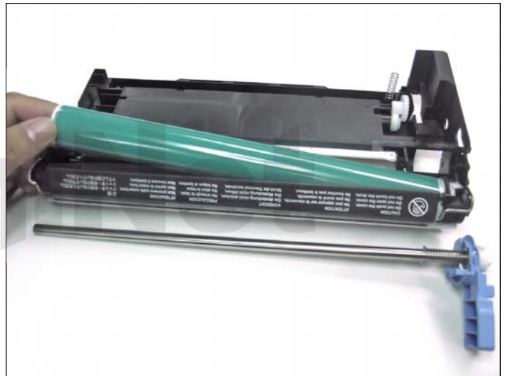
13. Carefully lift the drum out from the left side as shown. If the drum is reusable, set aside and keep away from light.
