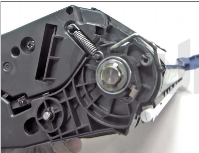
44. Install the drum cartridge tension springs.
