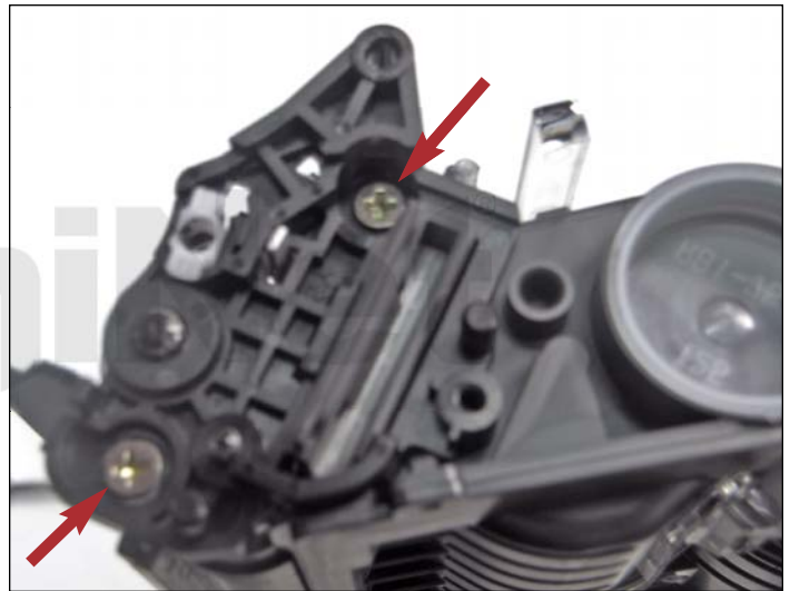
19. Remove the two Phillips screws from the roller support plate shown.
