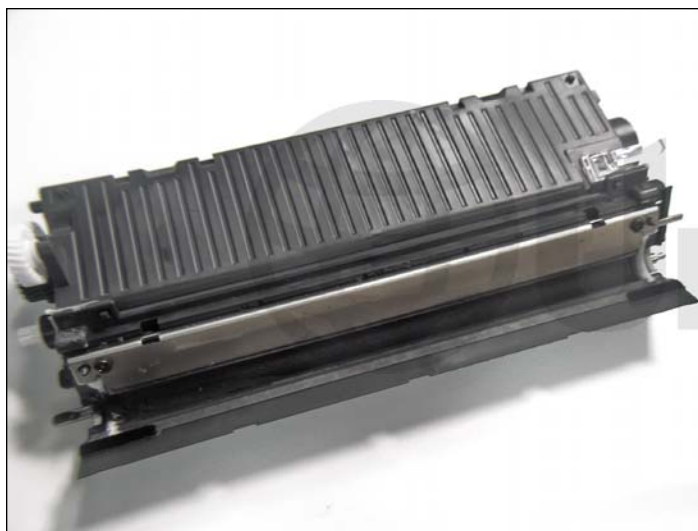
28. Remove the two screws from the doctor blade.
