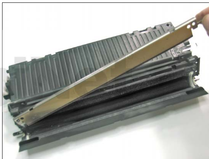
28. Remove the two screws from the doctor blade.
