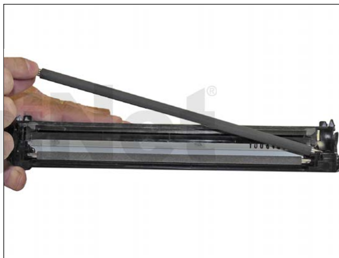
10. Remove the PCR from the assembly.
