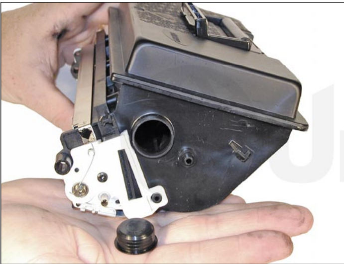
24. Remove the fill plug and dump out all remaining toner from the hopper. Vacuum clean.
