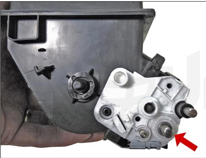
44. Install the bearing onto the developer roller shaft (gear side of the hopper).
