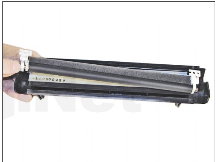
16. Pry up the white plastic holders and remove the PCR assembly.
