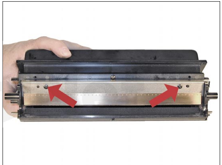
33. Remove the two screws and the doctor blade.
