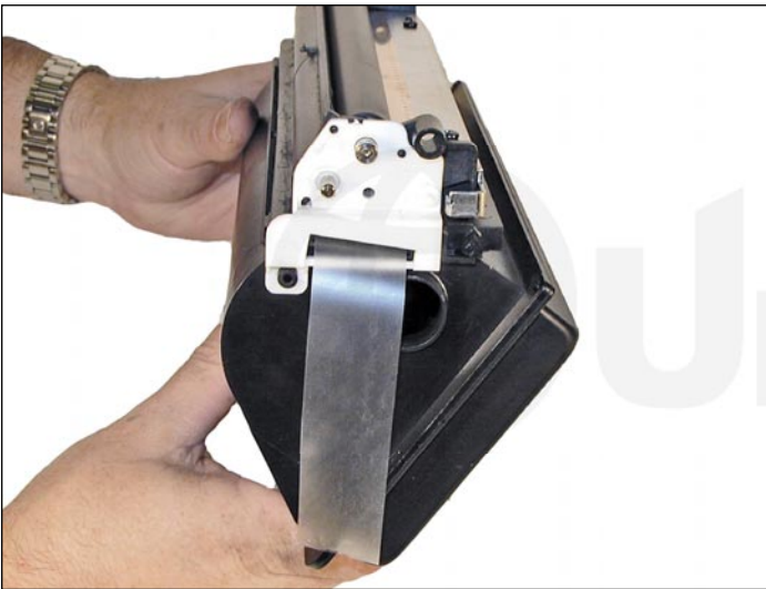
40. Install the white plastic alignment plate and the screw, on the fill plug side.
