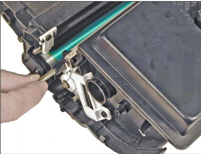
9. Slide the metal rod located above the developer roller away from the remaining end cap to free it from the end caps.
