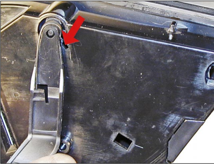
63. Install the drum cover arms. Place the arm into place and rotate the tail of the springs so they fit into their respective slots.
