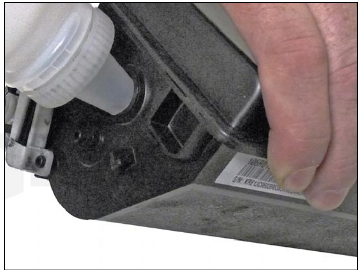
49. Fill the hopper with 3600 toner (330g for the 12k and 165g for the 6k). Replace the fill plug and check for leaks.
