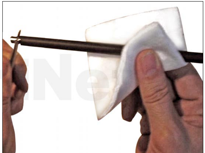
21. In case of contamination, clean with a small amount of water and mild soap. Otherwise, use a simple dry pad.
