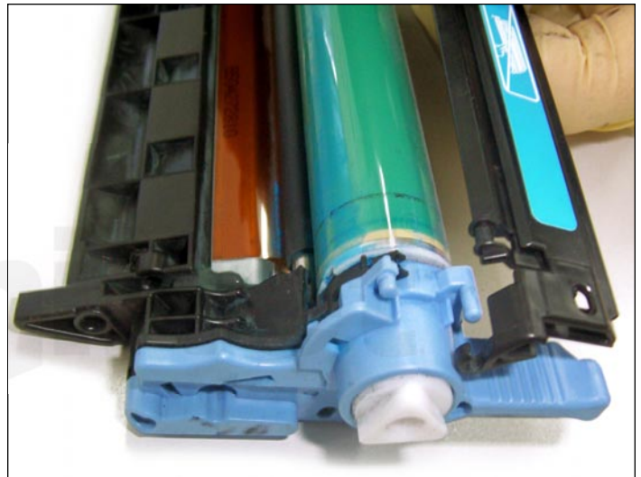
11. Unhook the drum shutter from the support tab on both sides of the drum unit.
