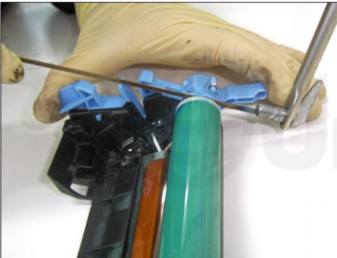
14. Carefully saw into the white plastic spindle and stop when it reaches halfway. Do not saw all the way through.
