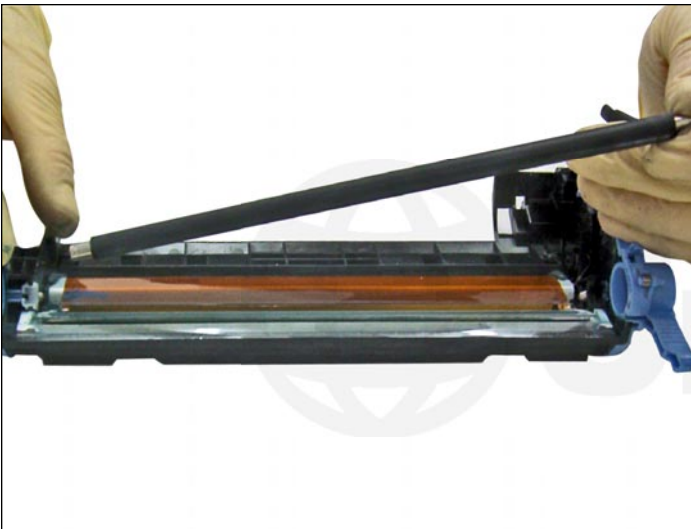
33. Slide the cleaned PCR into the saddle on one side, then place the other side using a pair of needle nose pliers.
