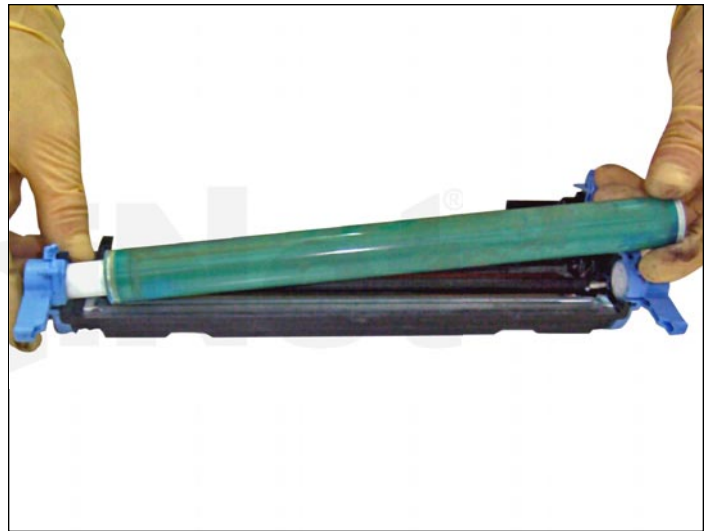
17. Carefully lift the OPC and slide it out in the manner shown.
