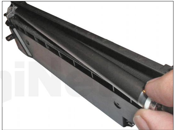
65. Install the developer roller with the gear-side first.
