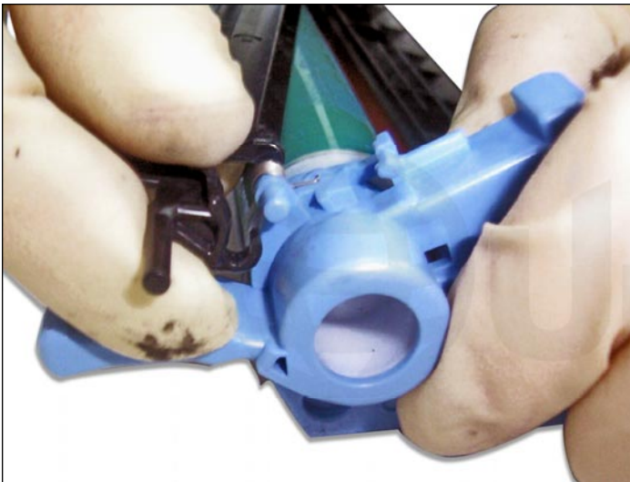
11. Unhook the drum shutter from the support tab on both sides of the drum unit.
