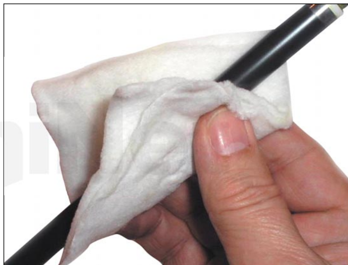
50. Secure the two bushings and clean the developer roller sleeve with compressed air. Alternate with a lint-free cotton pad. Be sure to clean the two bushings thoroughly.
