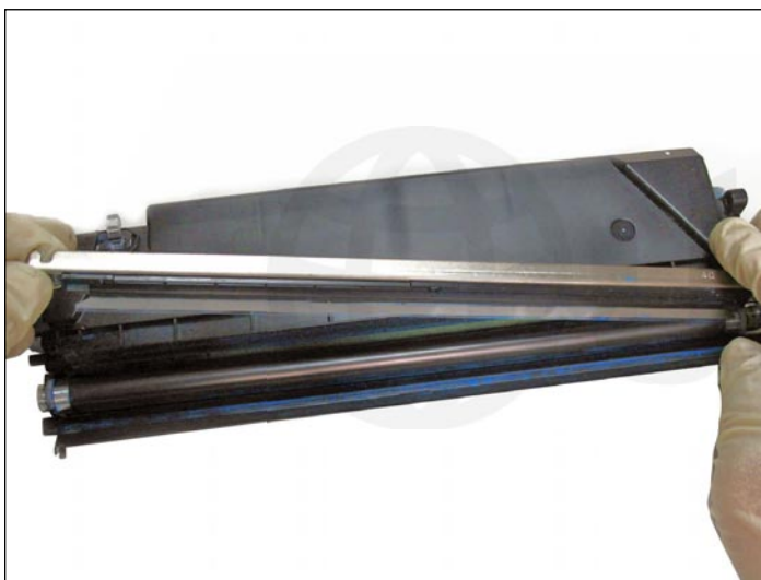
47. Carefully lift the doctor blade out as shown.
