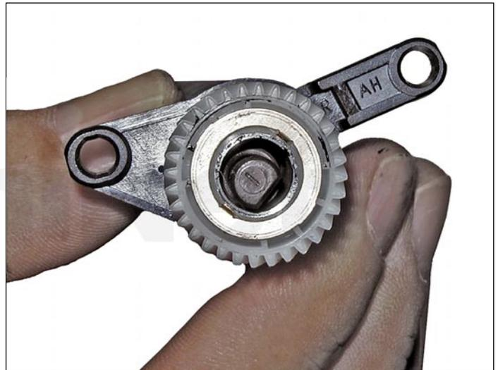
25. Install the magnetic roller drive gear and copper contact plate onto the magnetic roller assembly. Make sure the contact fits tight!
