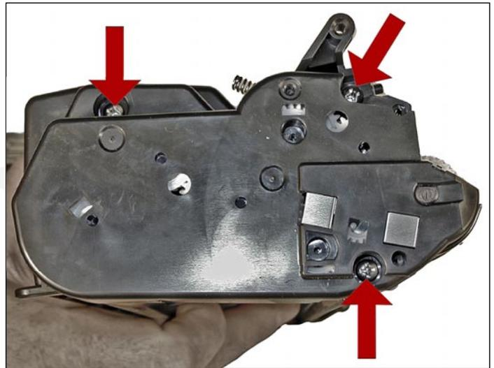
28. Install the gear end cap and three screws. If the end cap does not fit, the stationary magnet needs to be turned, so that it fits properly.
