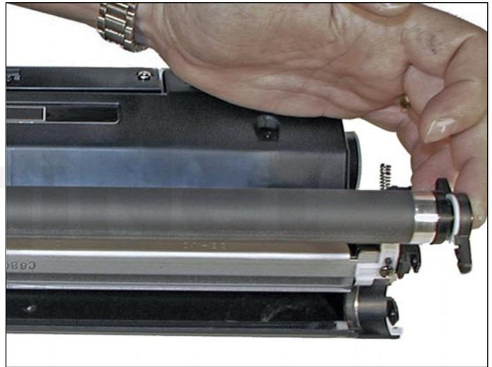
19. Remove the magnetic roller assembly from the cartridge.
