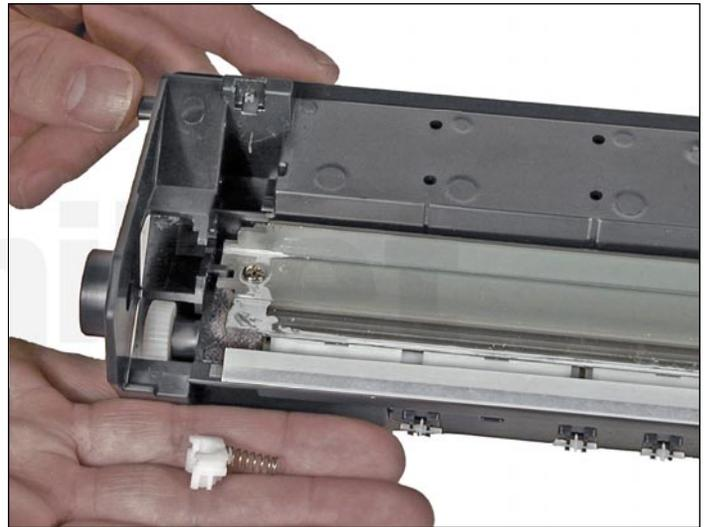
7. Remove the white PCR holder by carefully prying it off the cartridge. This holder must be removed to allow the wiper blade to be removed.
