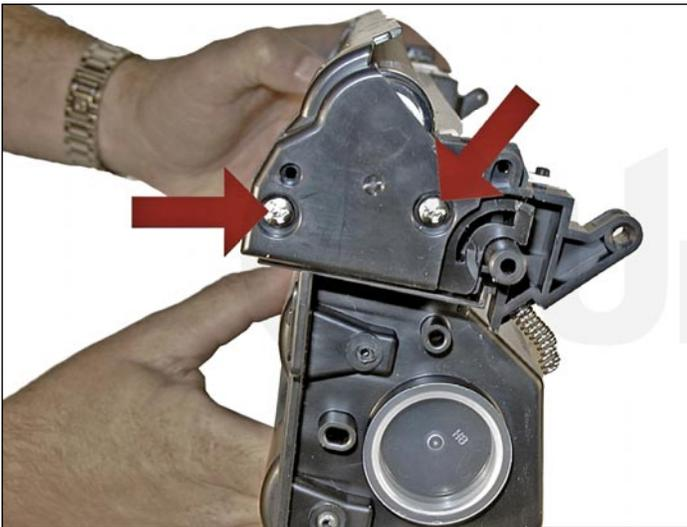
18. Remove the two screws from the small end cap on the left (non-gear) side.
