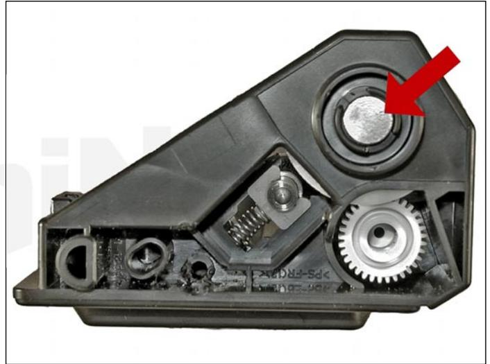
13. Replace the metal drum axle pin, and install it on the cartridge.
