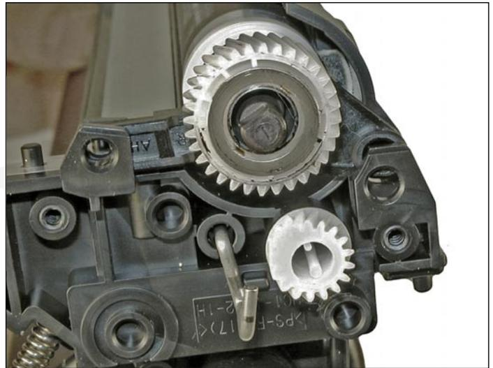
26. Install the magnetic roller assembly.
