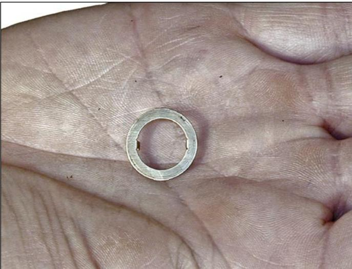
24. Clean the magnetic roller contact plate that you removed earlier from the drive gear. Clean the magnetic roller sleeve with a dedicated magnetic roller cleaner.
