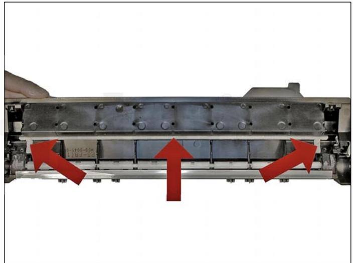
9. Clean out any remaining waste toner. Make sure the foam seals under the wiper blade are clean and not damaged.
