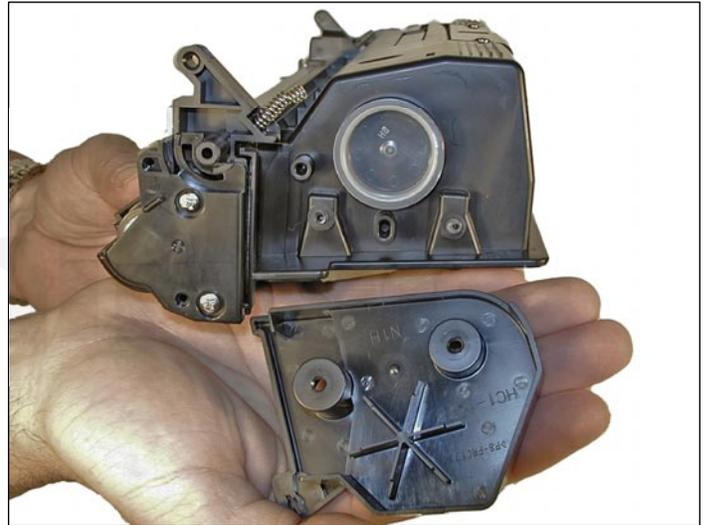
16. Take the supply section on the plastic end cap that is held on with plastic rivets.
