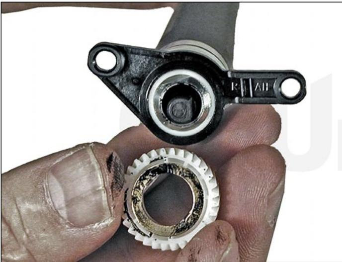
20. Remove the magnetic roller drive gear and copper contact plate, so they do not get lost.
