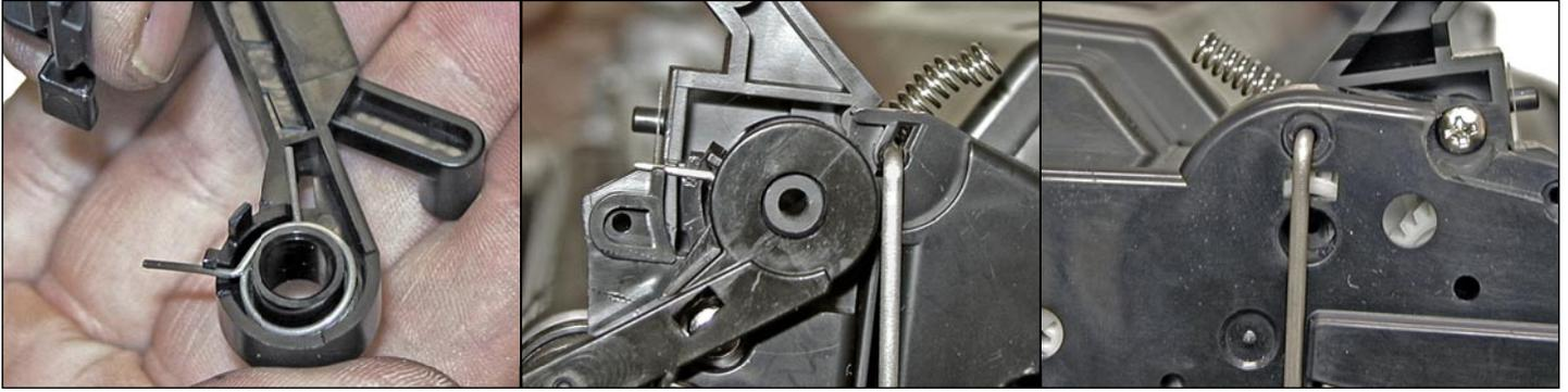
32. Set the spring on the drum cover arm as shown.
