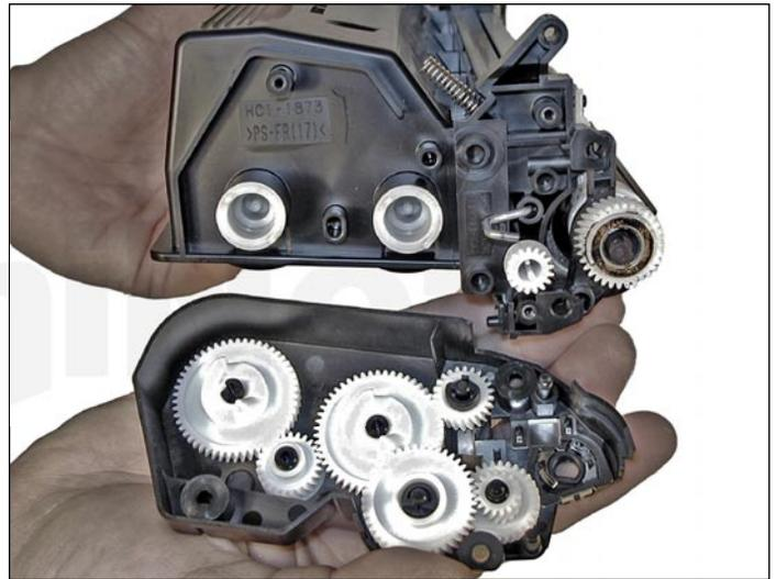
17. Remove the three screws on the large gear side end cap, and remove the end cap.
