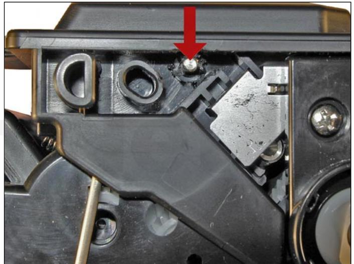
1. Note on each end of the cartridge there are small silver pins. To separate the two halves, these pins must be removed. There is no need to cut through the top of the cartridges to remove the pins. With a Dremmel tool or wire cutters, cut away the plastic from around the pins and remove the pins.
