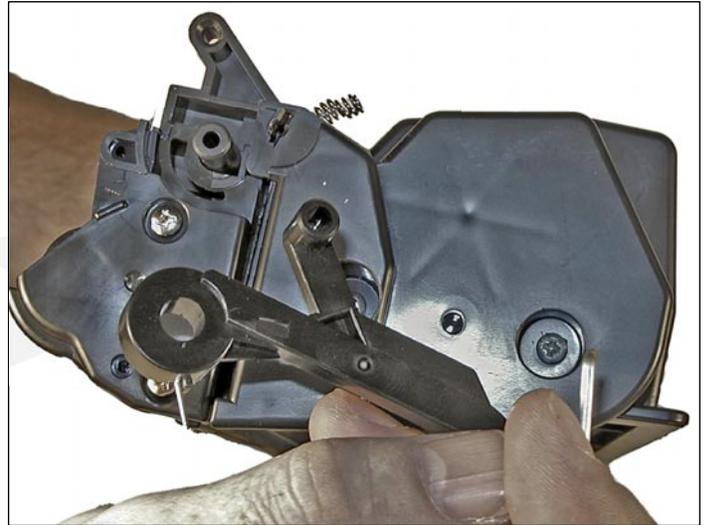
15. Remove the drum cover by prying up the metal bar on each side of the toner hopper.
