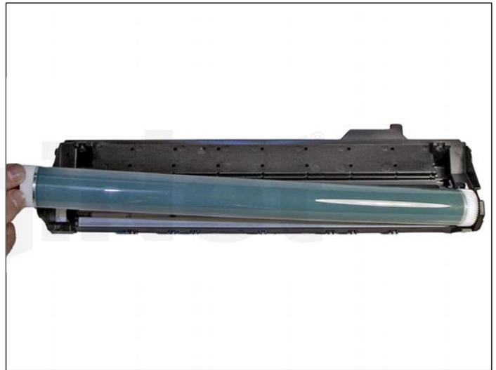
5. Remove the photoconductive drum, and place aside.
