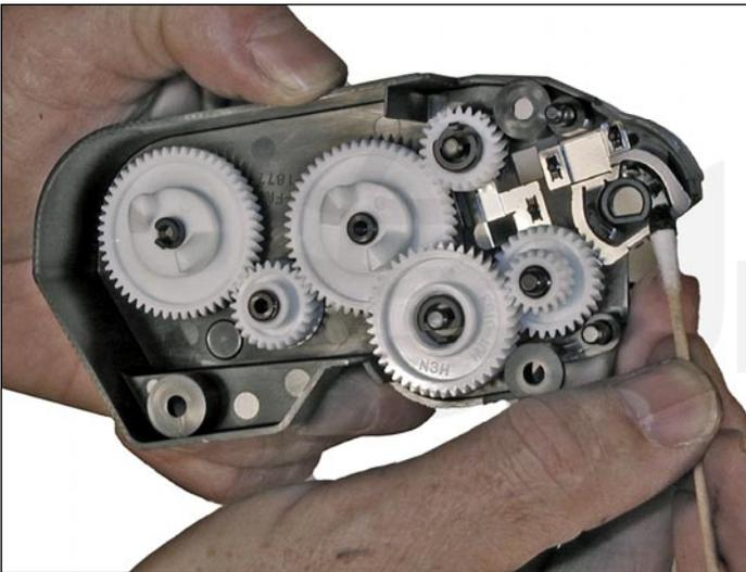
27. Clean the contacts on the gear end cap, and replace the conductive grease.
