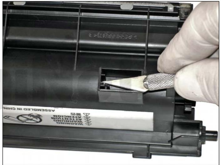
14. Using an X-Acto knife, carefully cut away the melted plastic tab.
