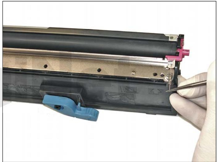
2. Using a hook tool, remove the two springs from the doctor blade. There is one at each end.
