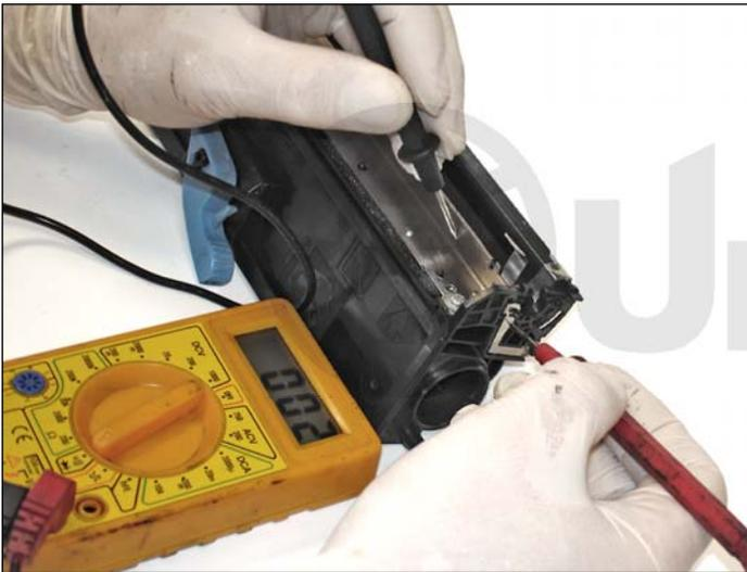
11. Use an electrical continuity tester to ensure good contact between the doctor blade and the main contact.
