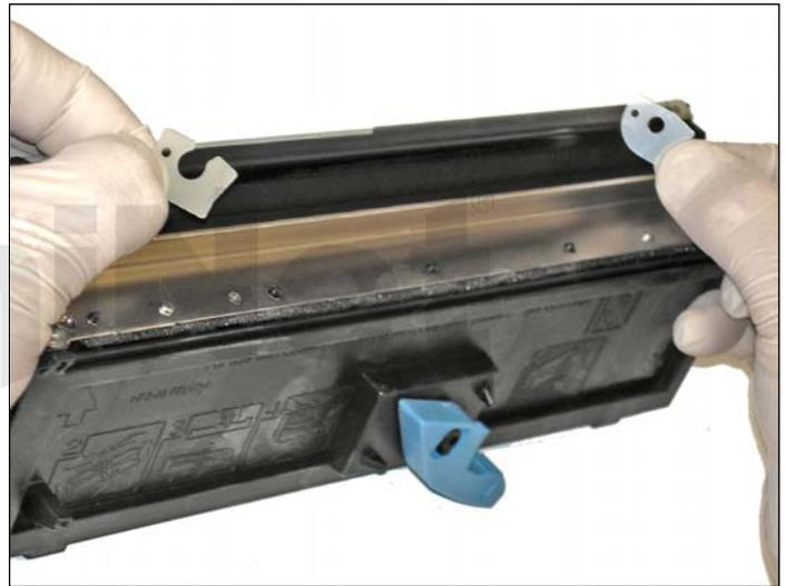
4. Remove the developer roller, lifting from the gear side first.
