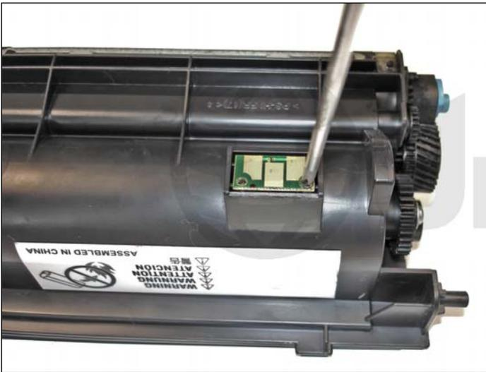
**REPLACING THE CHIP**
