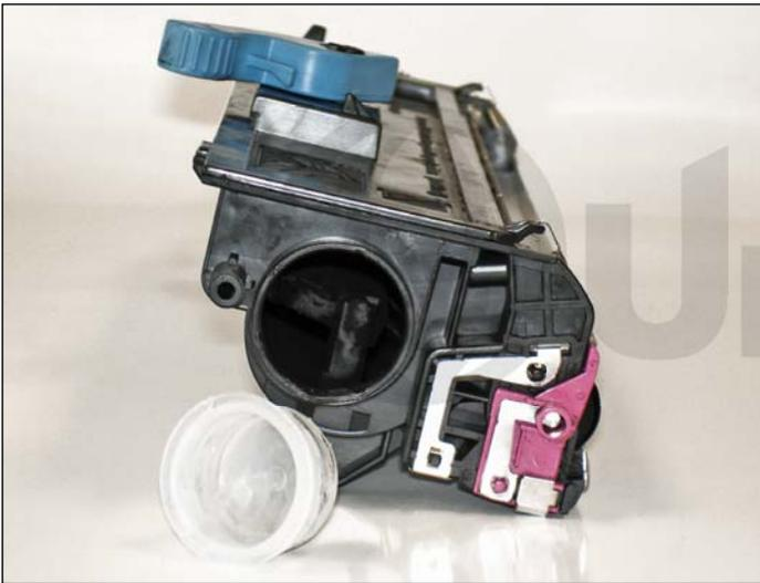
1. Remove the hopper fill plug and dump the remaining toner using compressed air.
