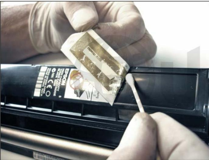
39. Remove the OEM label where the chip is placed as shown.
