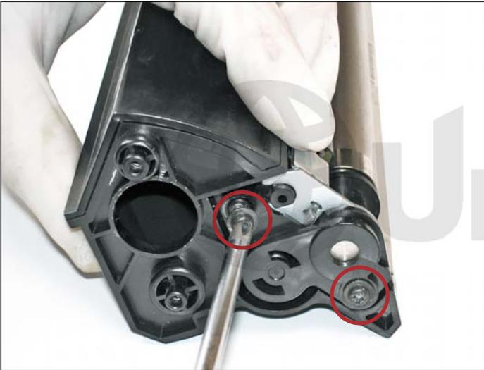
17. Remove the two black Phillips screws from the metal developer roller end plate shown.
