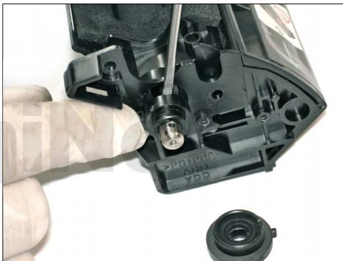
20. Remove the black adder roller bearings from both ends of the cartridge.
