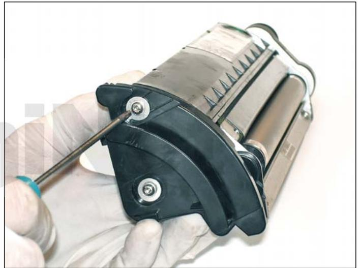
4. Remove the two torx security screws from the color cover side (gearless) using a security torx screwdriver.
