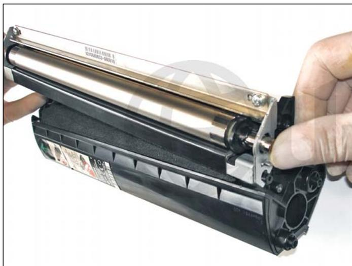
31. Install the entire developer roller assembly onto the cartridge. It should fit the previous position on the sealing foam.
