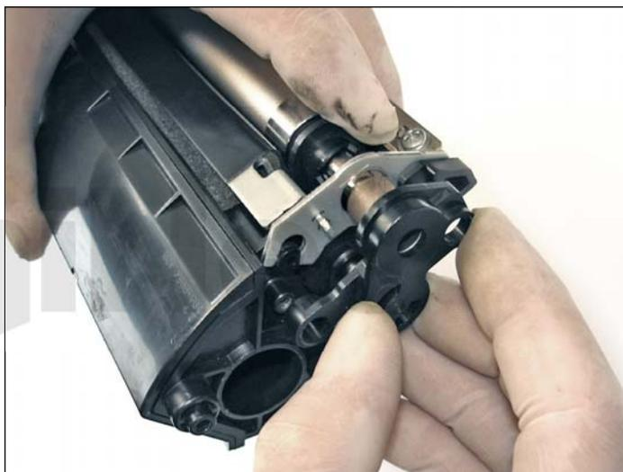
32. Place the black developer roller end cap on the right side as shown and install the two screws.
