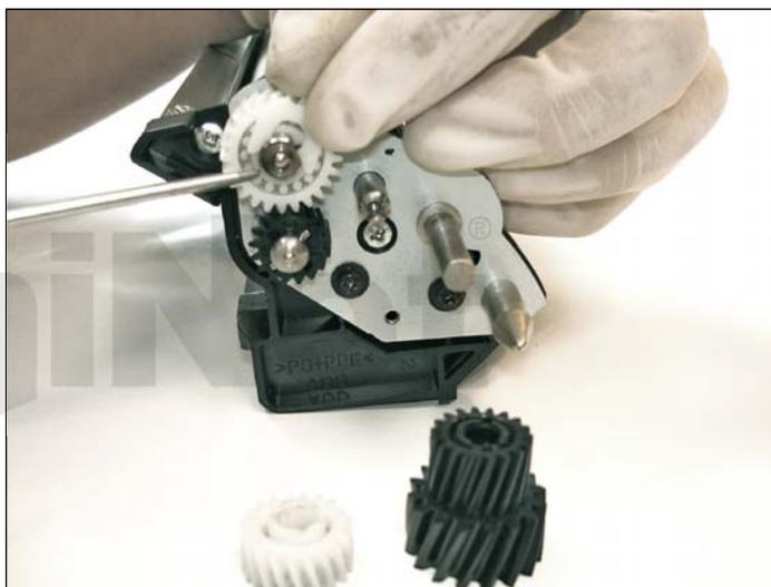
10. Remove the two loose gears shown. Carefully remove the white plastic U-clip from the upper developer roller guide gear as shown.
