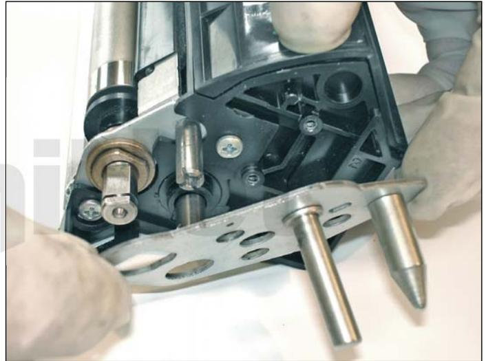
14. Remove the metal gear end plate.
