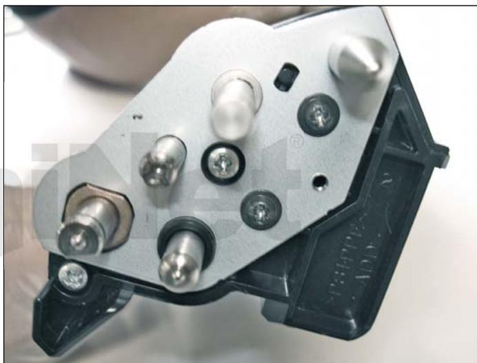
34. Place the metal gear support end plate in its proper fitting position with the previous the bearing installed.
