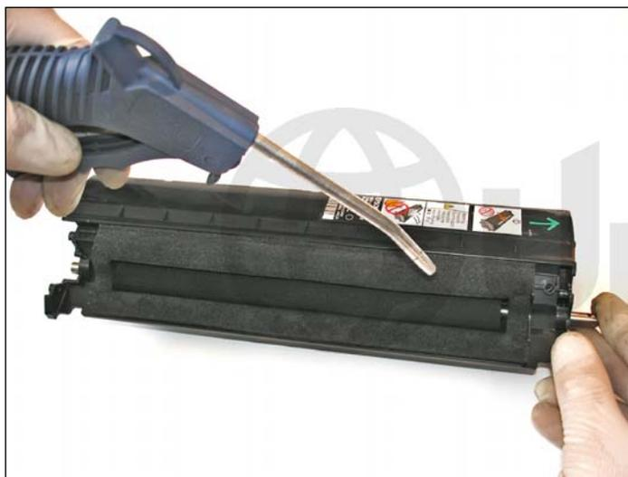
21. Use compressed air to clean the toner chamber and cartridge. Make sure the foam seal around the slot is clean and not damaged. Be careful to not damage the sealing foam.
