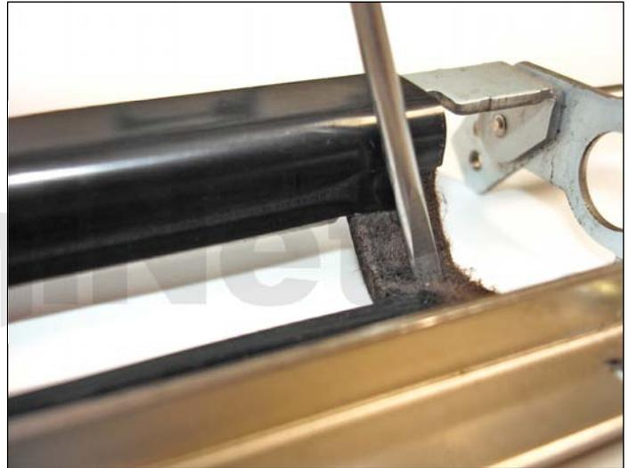
26. Comb through foams on both ends using a flathead screwdriver to prevent leaking. Make sure the foams and black mylars are in good condition, otherwise it can cause massive leaking. In case of toner adherence in the toner mylar surface, gently apply a cotton tip swap to eliminate all residual toner.
