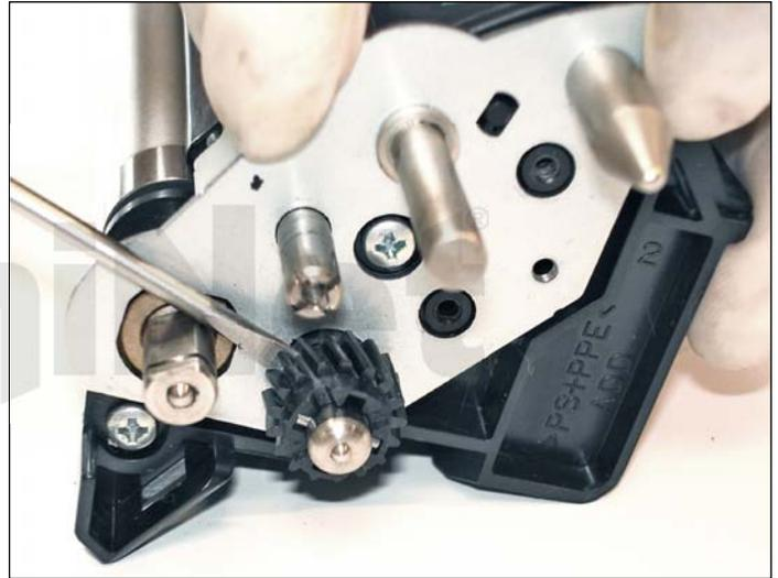
12. Carefully slide out the shaft using a flathead screwdriver between the black gear and the metal gear plate.
