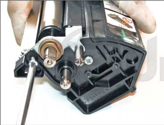
15. Remove the two Phillips screws which ensure the correct position of the developer roller frame. Note the thread is different.
