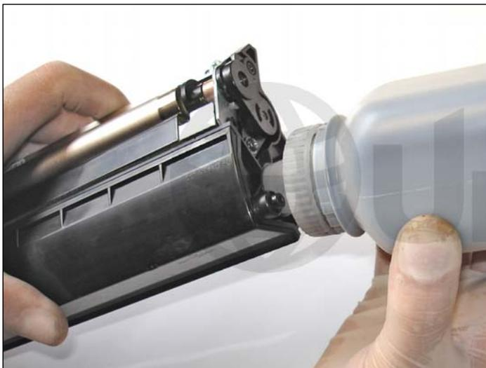
37. Fill the hopper on the gearless side with the appropriate amount of toner and install the fill cap.
