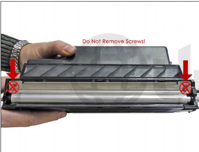
20. It is best not to remove the doctor blade as it is very difficult to get back in the right place. The entire magnetic roller section will be removed in the next few steps, so is possible to clean all the old toner/developer out.
