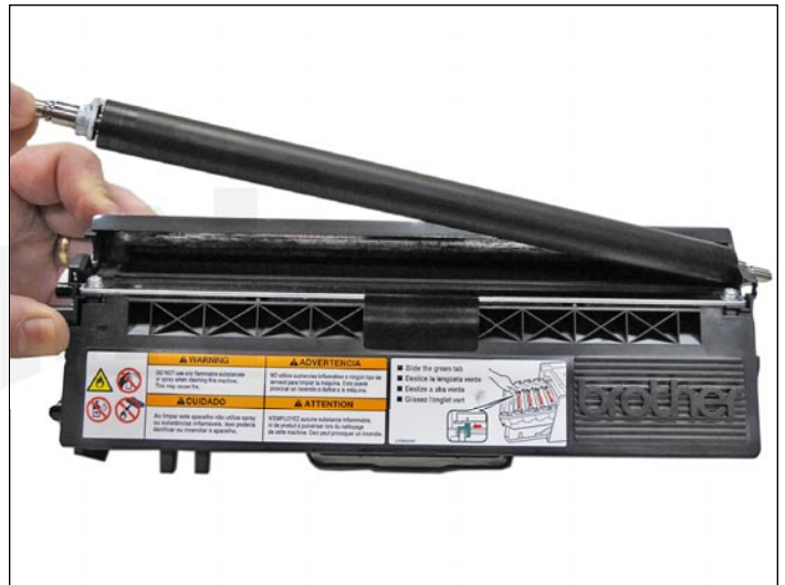
13. Remove the developer roller.
