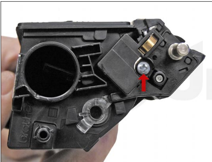
11. Remove the screw and contact side end cap for the developer roller.
