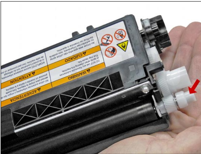
4. Pry off the white developer roller bushing.
