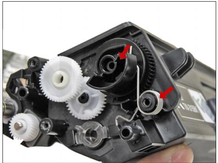
7. Remove the reset gear and spring.
