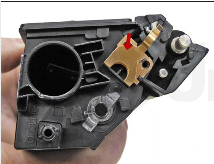
12. Carefully remove the copper contact.
