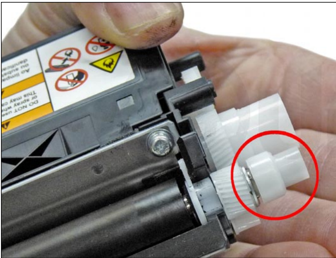
25. Install the developer roller bushing.
