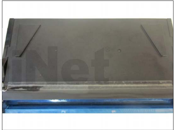
30. Install the cleaned doctor blade.
