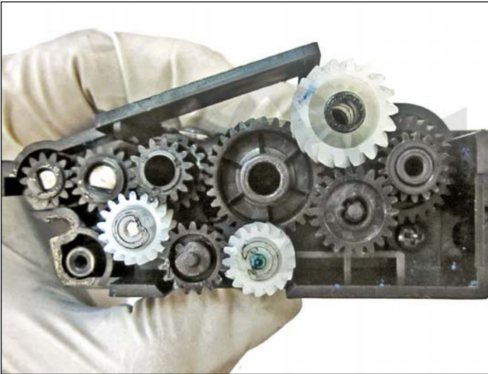
19. Remove the gears.
