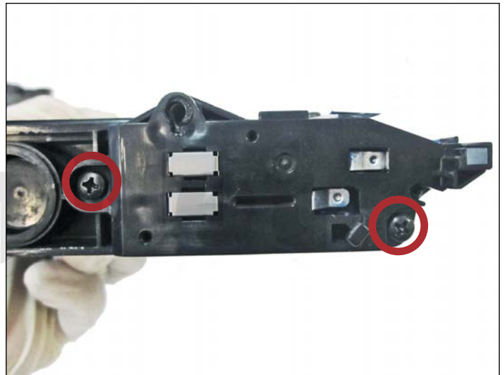
32. Install the contact end plate and screws.
