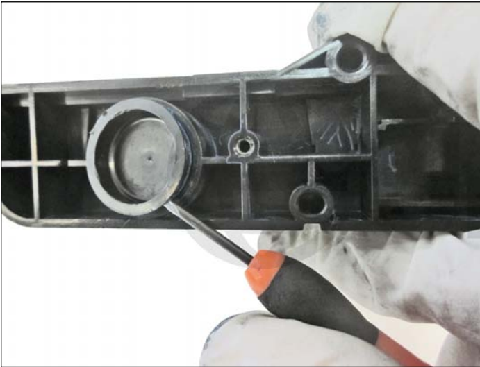
29. Remove the fill plug and clean out all remaining toner.
