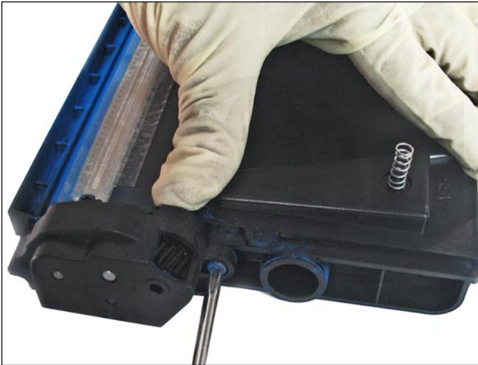
6. Remove the gear-side end plate screws, and the end plate.
