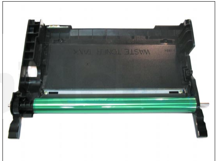
20. Always insert the drum axle through the non-gear side to install it. Inserting through the gear-side could damage the contact.
