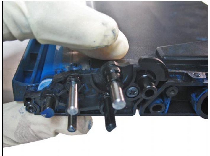
7. Remove the gears as shown.
