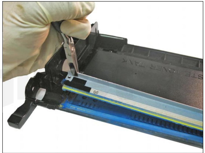
18. Lift the wiper blade out, using a pair of pliers.
