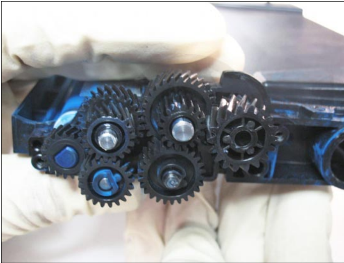
7. Remove the gears as shown.
