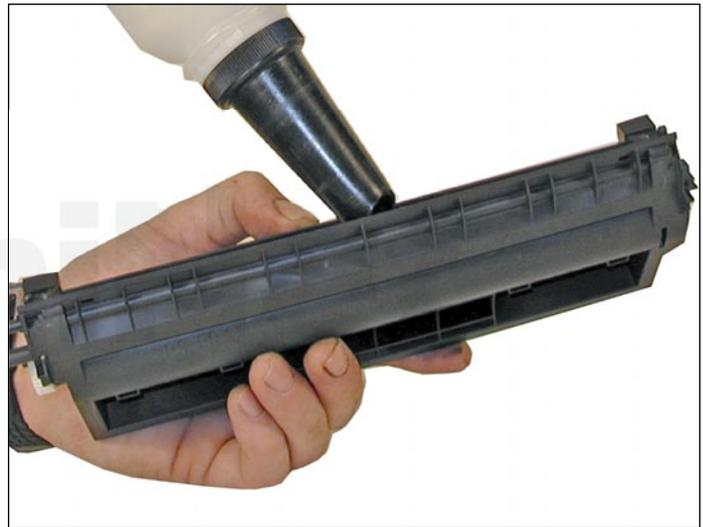
13. Fill through the magnetic roller opening with 190 grams of new replacement toner for use in HP 1200. You can fill through the fill hole, but until there is a seal available, you must hold the mag roller assembly in place (a tricky thing to do).
