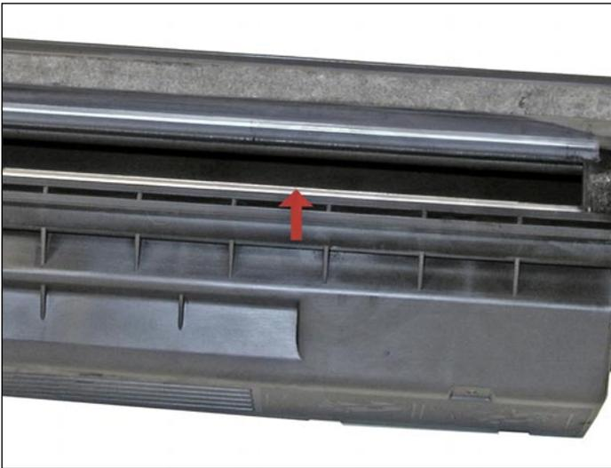
12. Once a seal becomes available, it should be placed on top of the silver areas shown. The seal tab fits through the right side of the cartridge (fill plug side).
