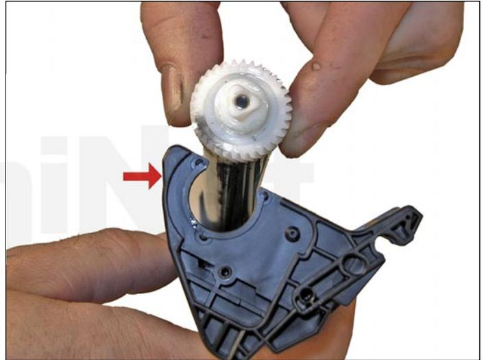
3. Remove the drum. Note the curved plastic piece around the drum. Because of this piece, the drum cannot be removed before the two halves are separated.
