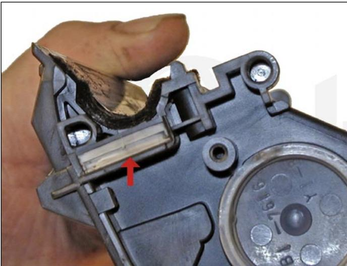
Shown here is a close up of the seal exit slot. Note that it has a rubber gasket that seals off the opening. This is a unique feature of this cartridge. Be careful not to tear the gasket when installing a seal!
