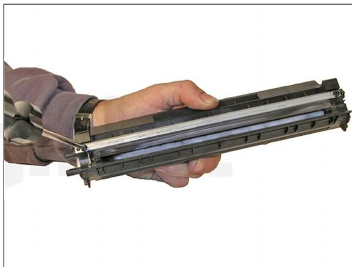
11. Remove the doctor blade. The HP 1200 doctor blade is almost identical to the AX except it is approx. 1/16" longer. Because of this a new blade is being developed.
