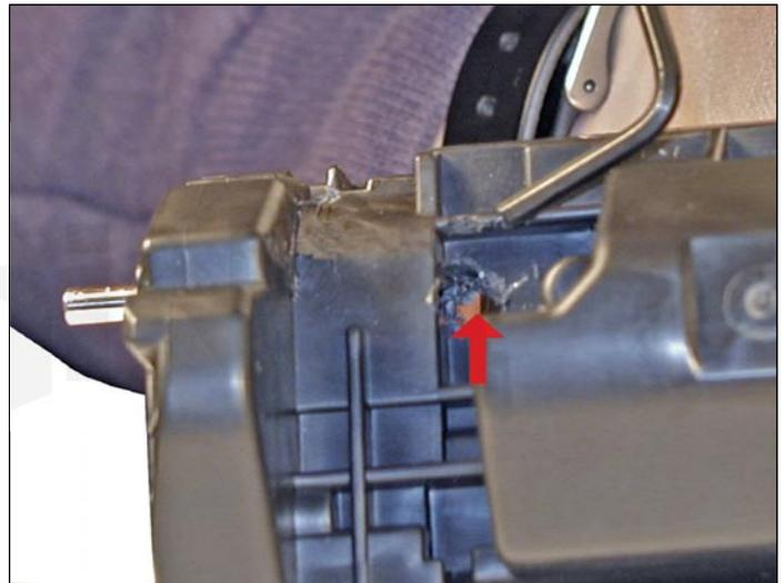
**Method 2:** Drill a shallow hole on each side of the cartridge as shown. Push the pins out with an allen wrench. Although this method also causes damage, you control how much there will be. This method is also safer for the PCR holder.
