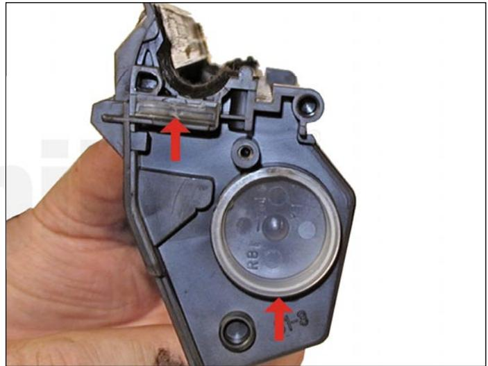
Shown are both the seal exit-slot and the fill plug.
