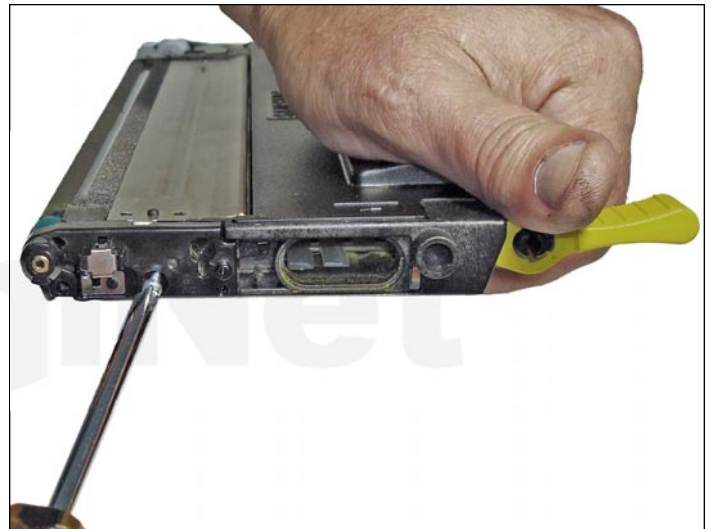
17. On the left side of the cartridge install the cover with the metal bushings properly lubricated with a small quantity of conductive grease and tighten with the screw.
