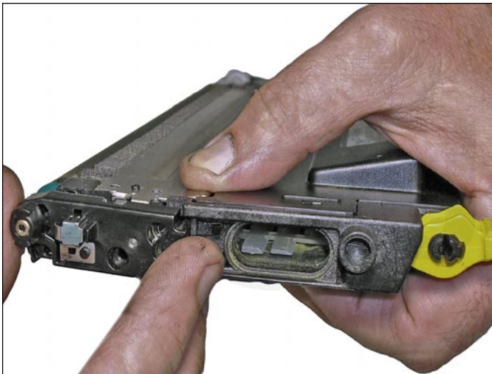
17. On the left side of the cartridge install the cover with the metal bushings properly lubricated with a small quantity of conductive grease and tighten with the screw.
