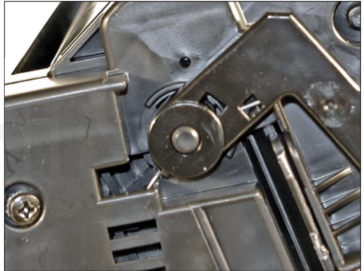
41. Install the arm onto the cartridge. Release the spring from the notch so that the tail fits as shown.
