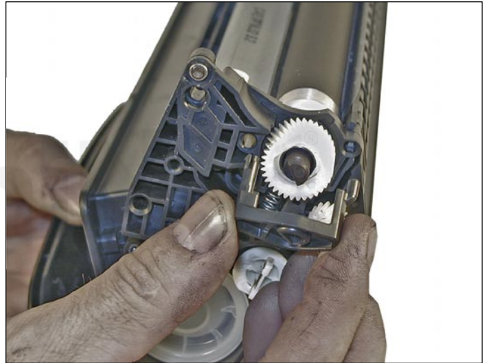
19. On the supply chamber, carefully pry off the magnetic roller (MRS) cover and remove.
