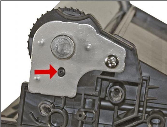
18. Install the drum, drum axle pin and screws. Make sure that the plastic pin is centered in the oblong hole of the metal axle pin (just like the HP 4000 cartridges).
