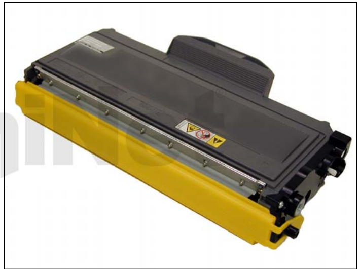
19. Install the developer roller cover.
