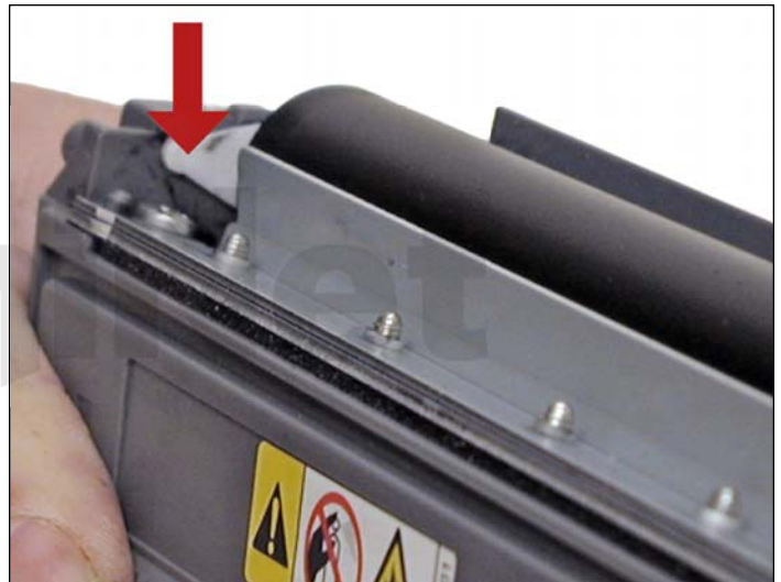
9. On the gear side of the developer roller, press in on the locking tab and rotate the developer roller lock up.
