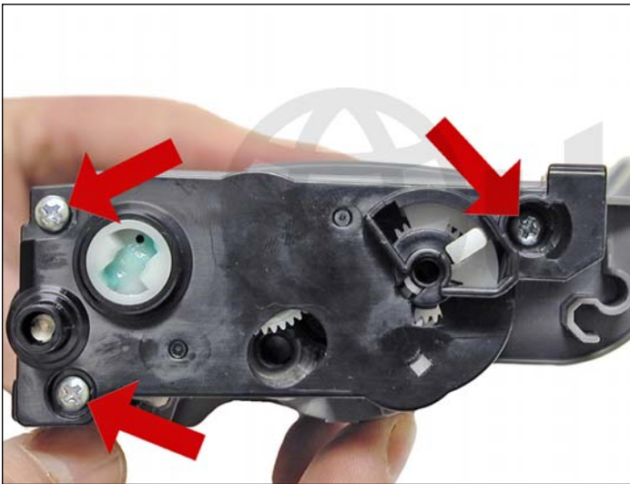
16. Install the gear cover plate, and three screws.
