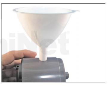
9. Insert a funnel through the hole. Be sure to shake the toner bottle well before opening. Pour the appropriate amount of toner via the funnel.
