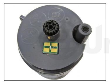
12. Peel off the strip to expose the adhesive on the reverse side of the new hardware replacement chip. Install the new chip in the small space shown. Remanufacturing complete.
