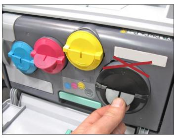
6. Do not drill or place any seal or adhesive on/near the top area of the cartridge. The space between the top surface of the cartridge and the housing wall just above it is very tight. Friction or rubbing while inserting the cartridge can cause the seal to loosen or break off and lead to toner leakage.
