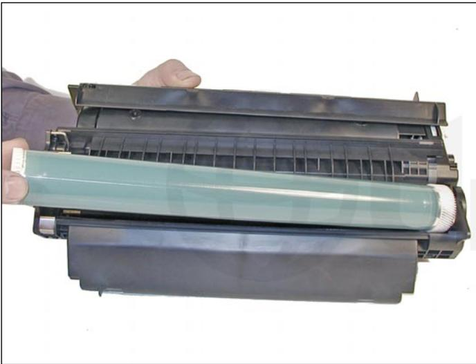
3. Remove the Photoconductive drum, being extremely careful not to scratch it. If the drum is in good shape and you plan to reuse it, blow off any toner and debris from drum being careful not to let the air gun come in contact with the drum surface. Do not polish or wipe the drum with a dry cloth since this may scratch the drum.
