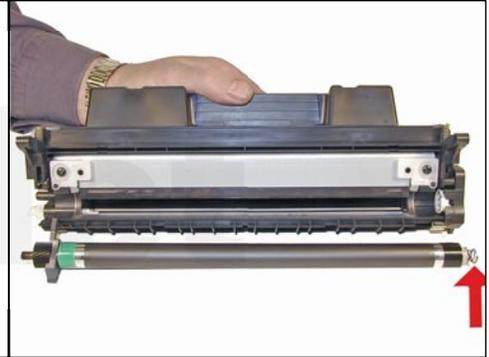
8. To remove the magnetic roller, first remove the right end cap by removing the two screws. Note the gears in the end cap are held in place. Carefully lift the roller out of the cartridge. Be very careful not to damage the wire contact at the opposite end of the roller.
