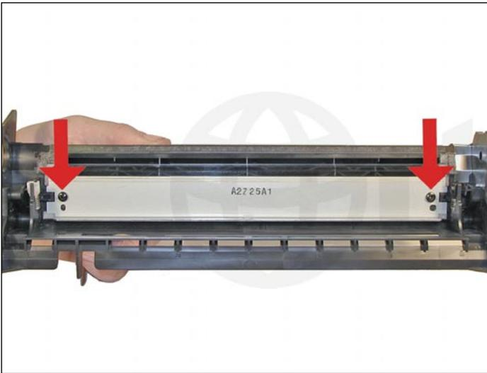
6. Remove the two screws and the wiper blade, and clean the toner out of the waste chamber.
