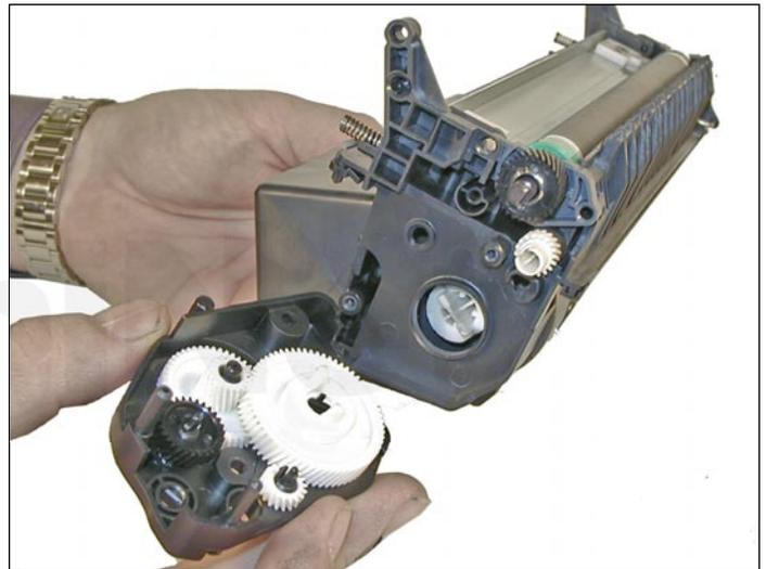
17. Install the large end cap and two screws.
