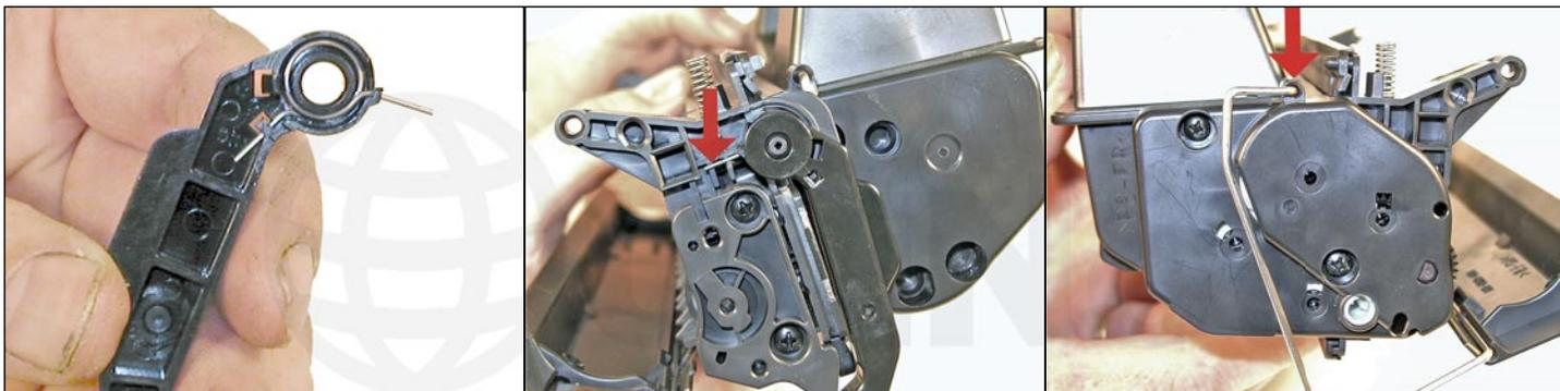
22. Install the drum cover onto the toner hopper.
