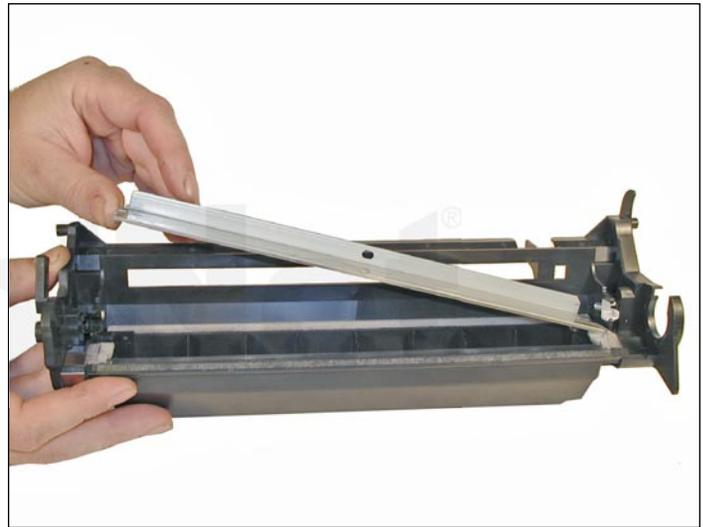
7. Due to the aggressive nature of the toner used in these cartridges, we recommend that the wiper blade be replaced each cycle. Lightly coat the new blade with Kynar drum padding powder. Replace the wiper blade into the cartridge.
