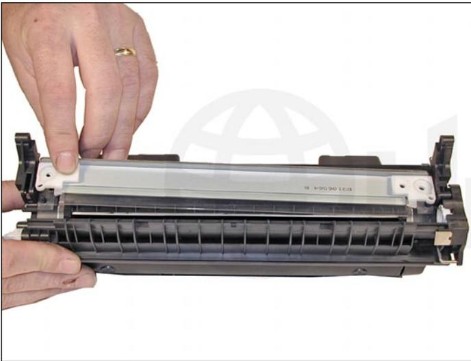
14. Install the new doctor blade. If the clear spacers are lost, make sure that the new blade came with them attached. Conversely, if the new doctor blade has spacers, make sure that you remove the OEM spacers. Only one set of spacers should be installed!
