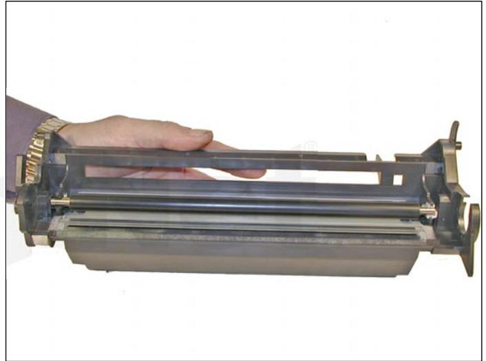
19. Replace the cleaned primary charge roller.
