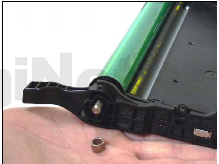
10. Remove the metal bushing.
