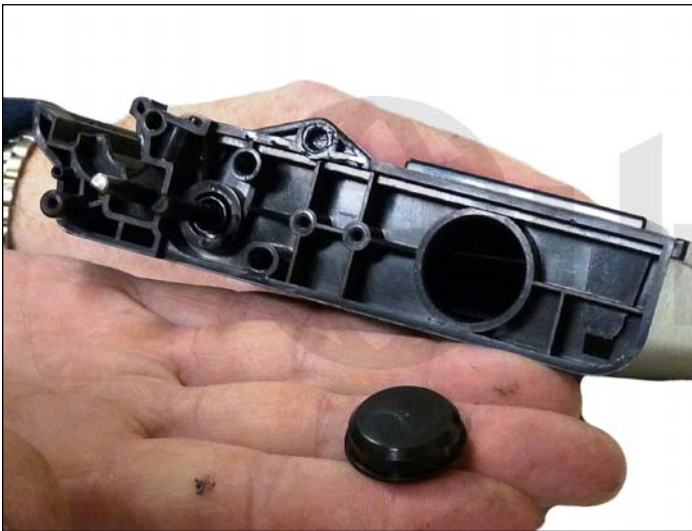
29. Remove the fill plug and clean out all remaining toner. Pay special attention to the feed roller. Any buildup here will cause streaking later on.
