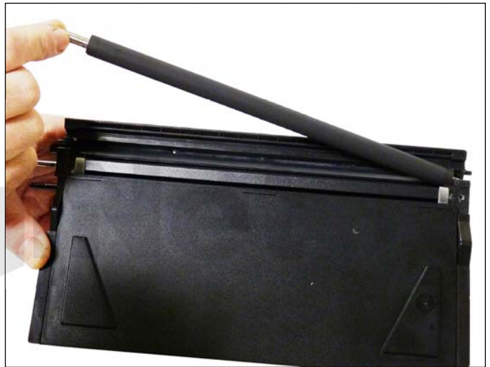
28. Remove the developer roller.
