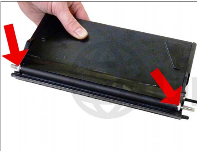
31. Install the developer roller and two bushings.
