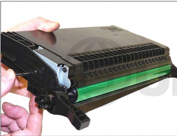
39. Install the two metal hinge pins, long pin to the drive gear side.
