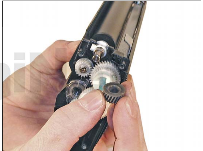
8. Remove the E-Ring and small gear.
