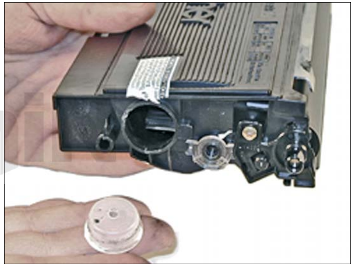
2. Remove the fill plug from the toner cartridge. Dump the remaining toner and vacuum/blow out the cartridge. Make sure that the gear area is clean. Leaving any toner in the teeth of the gears may cause a tooth to be damaged and cause a clicking noise. We have found it best to use compressed air to clean them out, but to also keep one hand over the gears to protect them.
