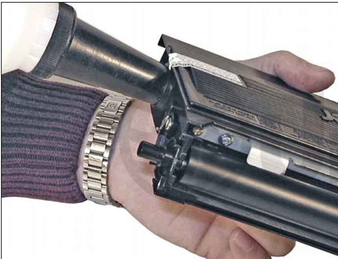
18. Fill the cartridge with toner for use in Brother 2030.
