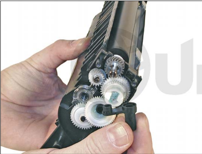
7. Remove the black plastic spacer from the developer roller shaft.
