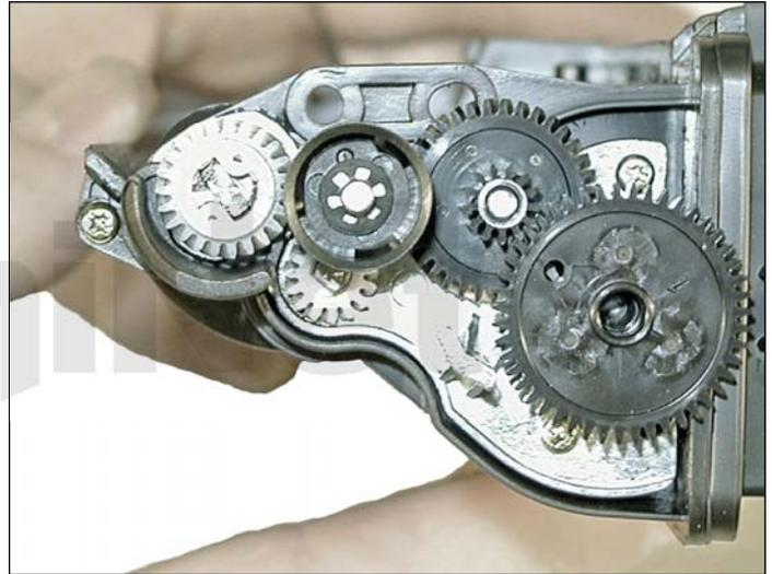
19. Install the gears. The large gear with the long shaft fits onto the toner agitator bar inside the hopper. Spin it a few times and listen to make sure it is engaged properly. On the large drive gear, make sure the flat washer is in place, and install a new star lock washer. Make sure the lock washer is pressed down fully against the base of the gear.
