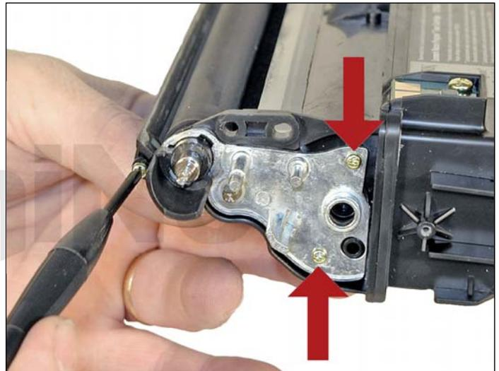
18. Install the gear axle plate and three screws.
