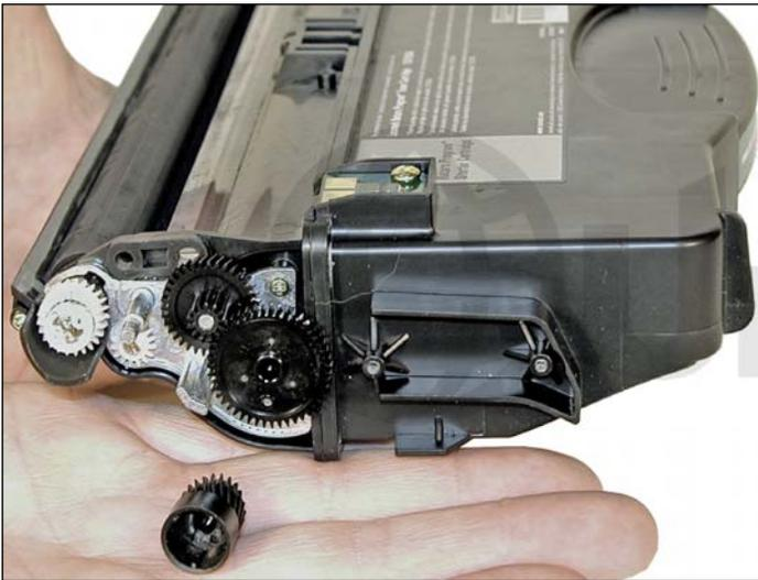
8. Remove the large black drive gear. Make sure you don't lose the small flat washer from under where the star washer was.
