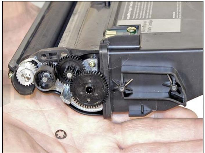
7. On the large black drive gear, there is a locking star washer pressed onto the shaft. With a small pair of wire cutters, cut the old washer off, and remove. You can try to bend up the different legs of the washer, but that is very time consuming, and most likely at least one leg will break anyway and the washer will still have to be replaced.
