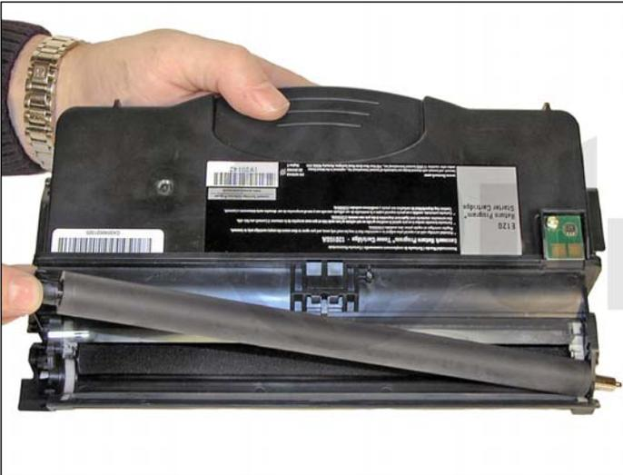
14. Lift the developer roller out of the cartridge.
