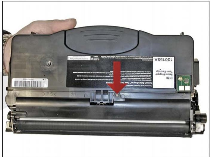
23. Install the developer roller cover and screw.
