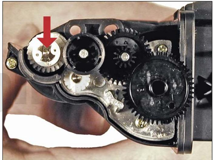
9. On the white developer roller gear, take the tips of your small wire cutters, and place them into the two small holes.
