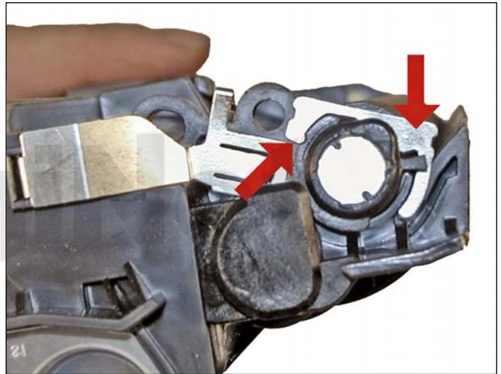
16. Reinstall the developer roller. Spin the plastic bushing so it is locked in place.
