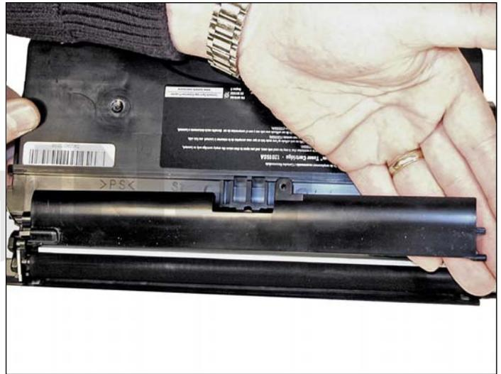
4. Lift up the developer roller cover from the center, and remove.
