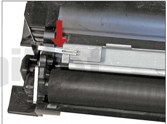
21. Clean the doctor blade and install. Make sure the metal tab on the right side fits into its slot.
