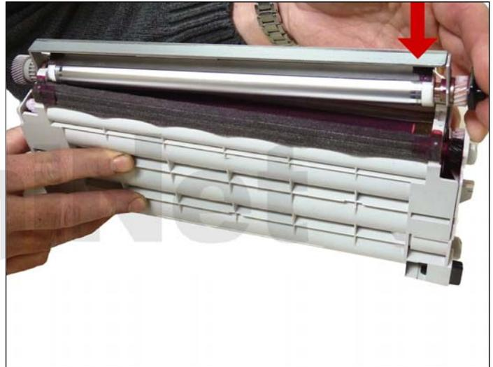
2. Lift up on the doctor blade side and remove the developer roller assembly.
