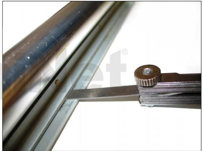
6. It is best not to take the doctor blade assembly apart, but if you do, use a gapping gauge to measure the gap by each of the five screws before removing any of them. Set the gap back to the proper distance when re-assembling the blade assembly.
