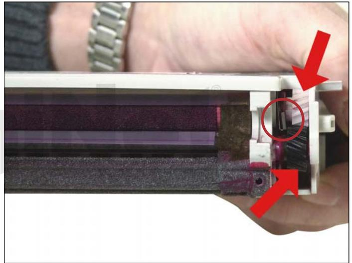
4. Make sure the gears on both sides of the cartridge are clean and turn freely.
