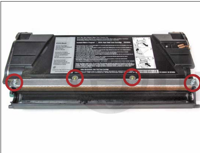
10. Remove the four screws shown that hold the doctor blade in place. Note the location of the doctor bar. It must be positioned in the same manner for reassembly.
