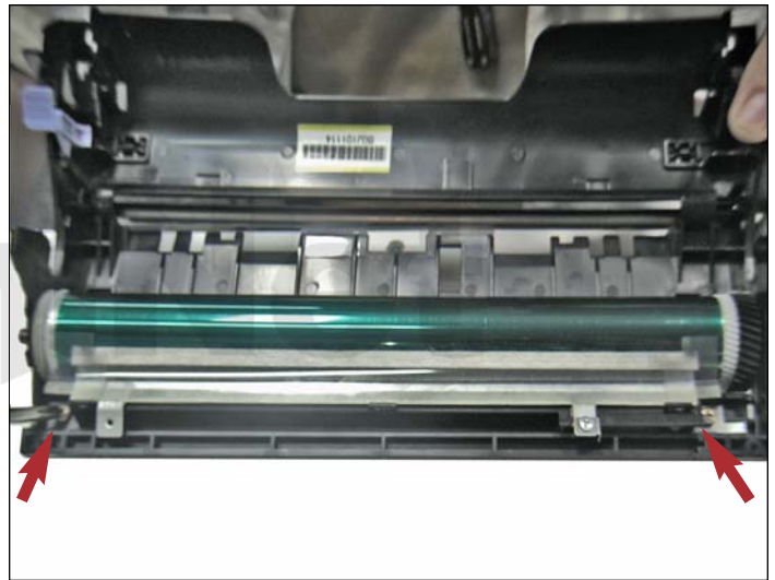
16. With a Phillips screwdriver remove the two screws holding the drum cleaning assembly. You will notice that it contains a cleaning felt, recovery blade and a couple of scraper blades.
