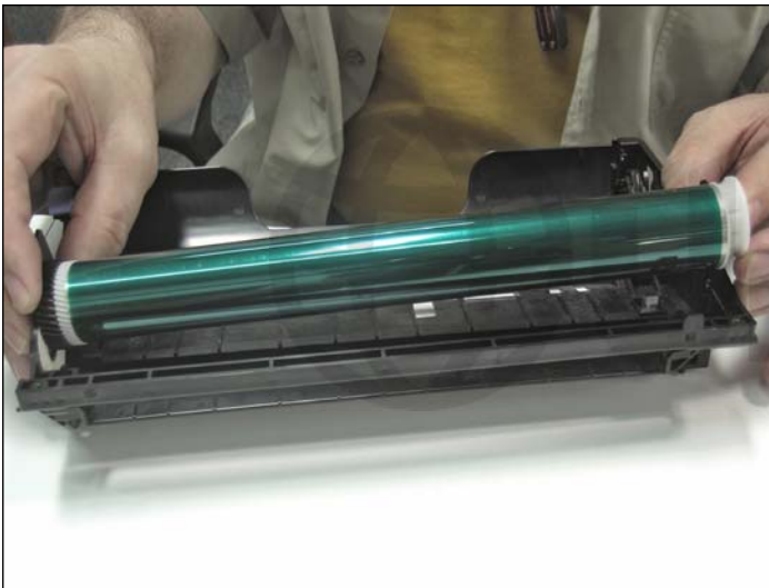
21. Remove the drum. There will be a spring-loaded clutch piece at one end, and a drive gear on the other side that will come loose.
