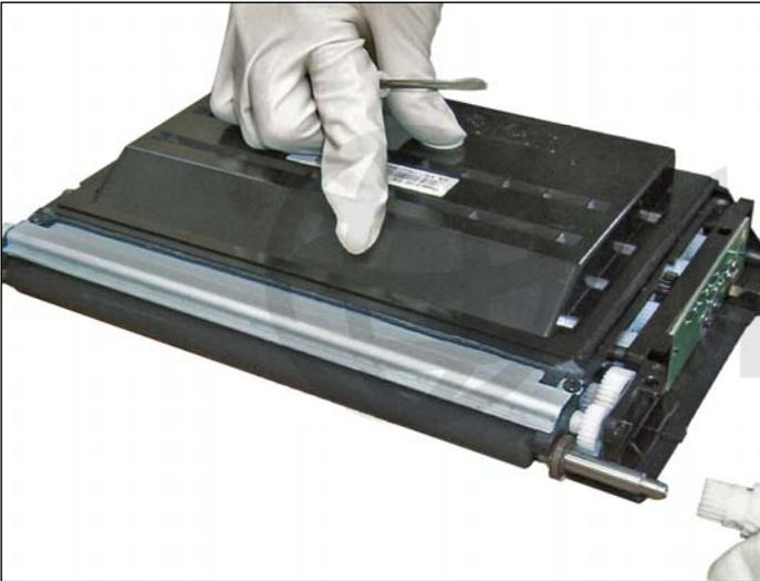
5. Remove the loose gears from each side.
