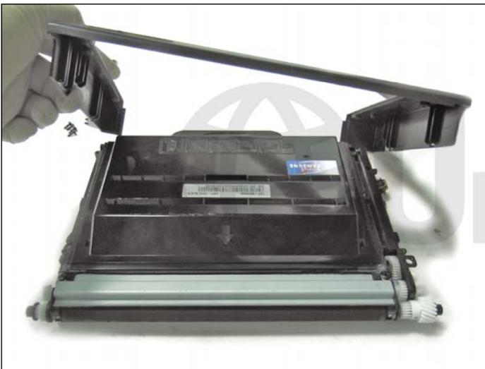
3. Remove the outer shell cover. You will notice a small adhesive holding it in place. Removing the cover should not affect it.
