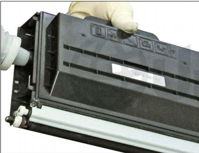
9. After thoroughly cleaning the cartridge and reinstalling the cleaned components, you are ready to fill with appropriate aftermarket toner.
