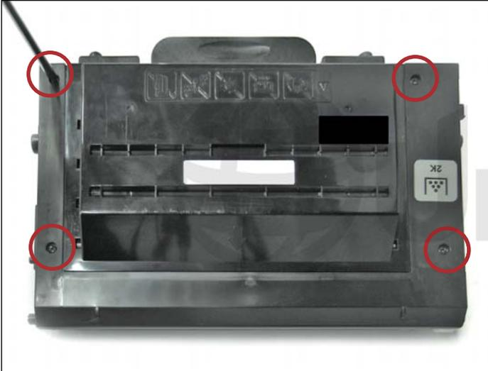
1. Remove the four screws from the top outer shell cover of the cartridge.
