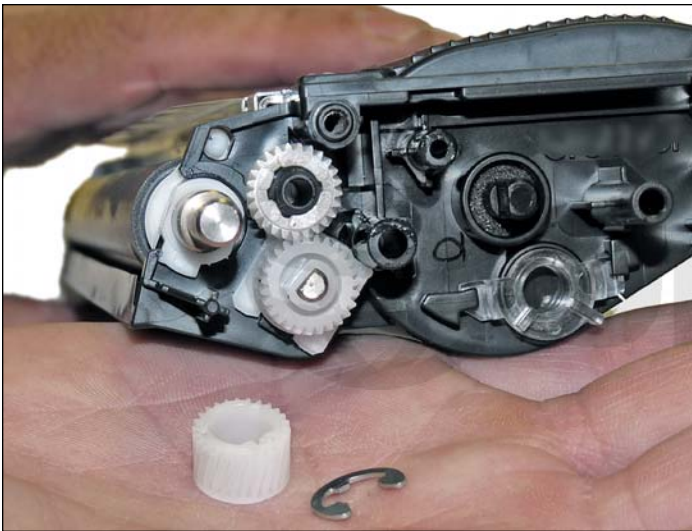
6. Remove the E-ring and developer roller gear.
