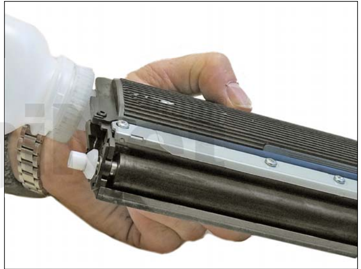
22. Fill the cartridge with the appropriate color and amount of toner for Brother HL-3040/TN210.
