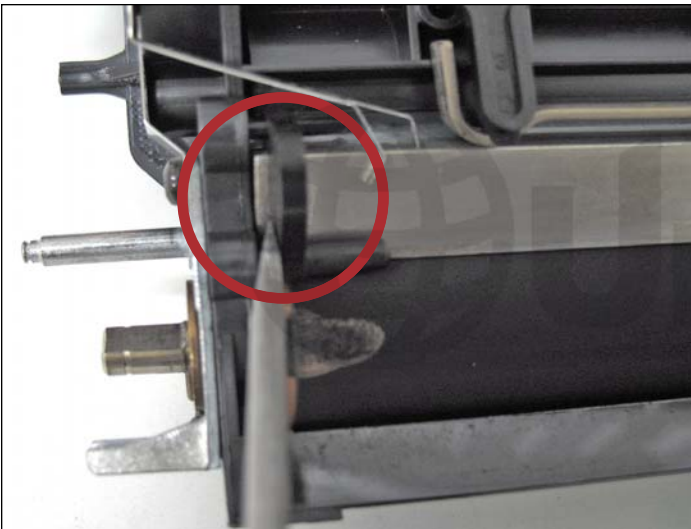
21. First, slide out the retaining tab (shown) that holds the doctor bar in place.
