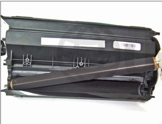
29. Finally, remove the developer roller as shown.
