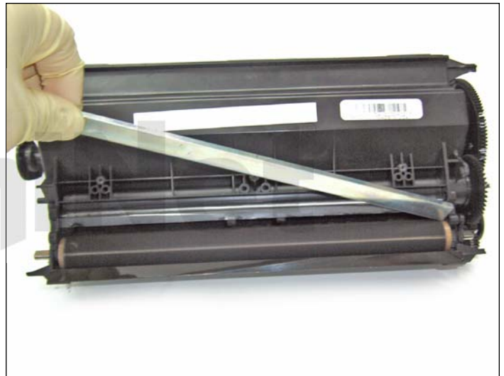
22. Remove the doctor bar as shown.
