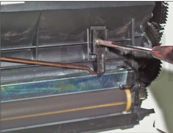
19. Remove the leaf spring positioning holder by removing the screw that holds it in place.
