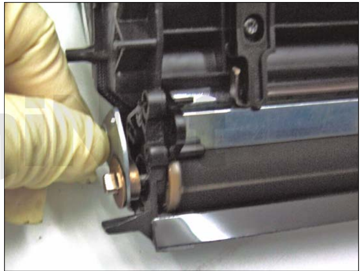
16. Now, remove the gear support plate by sliding it out.
