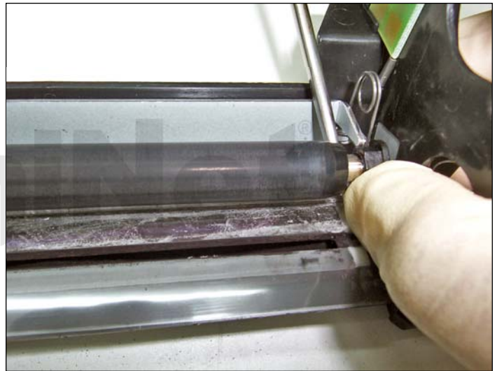
36. Pry out the PCR together with the PCR saddles.
