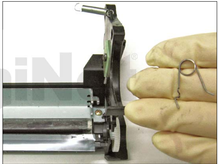
38. Once the PCR has been removed, the PCR spring (shown) can then be released.
