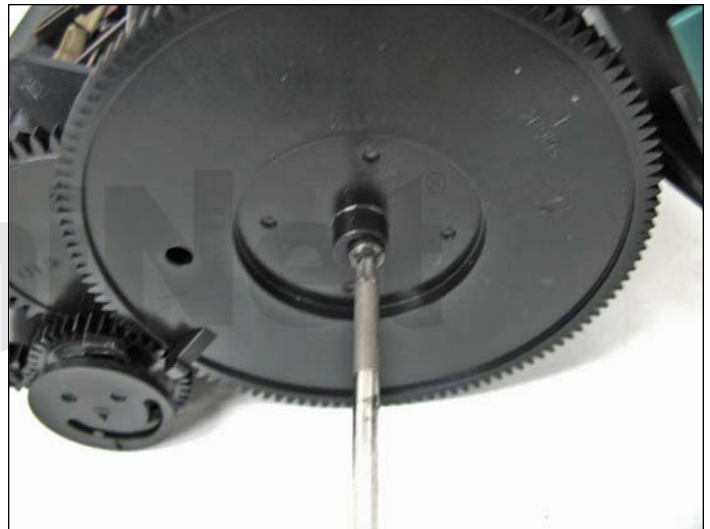
30. To access the fill plug, you must first remove the toner agitator drive gear using a star tool.
