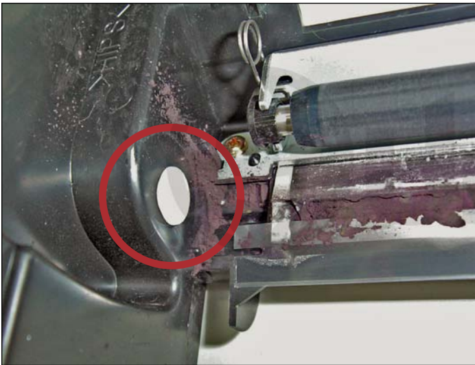
35. Notice the white plug (shown magnified). If removed, toner from the waste hopper would leak. Remove during cleaning.
