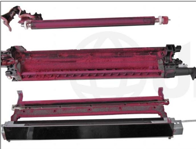
20. Clean the disassembled developer section with a vacuum.
