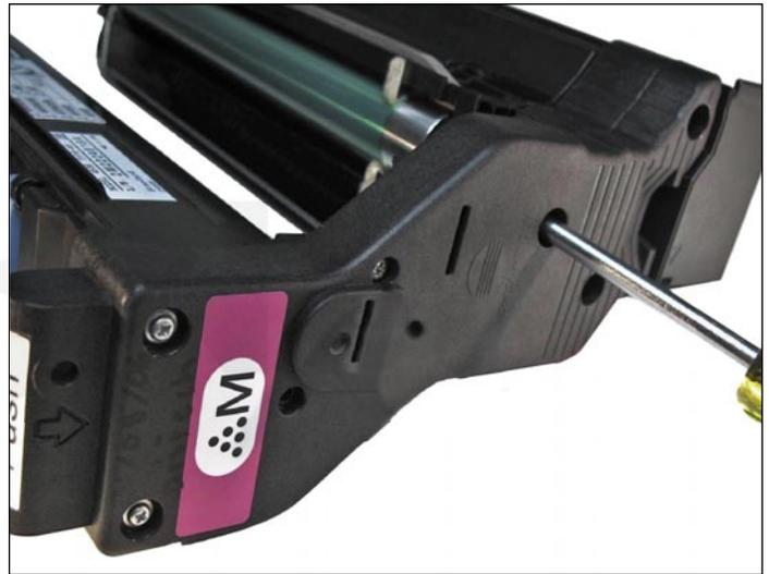
53. Secure the outer end cap with the seven screws.
