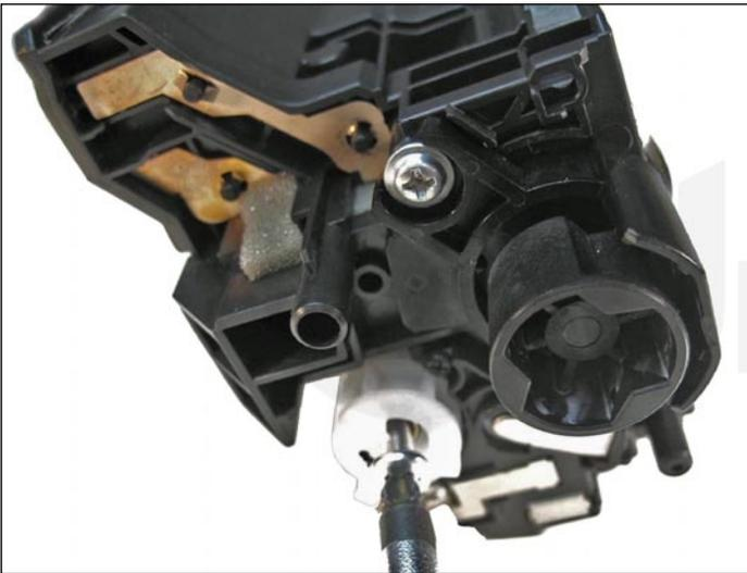
43. Install the developer roller drive gear and screw.
