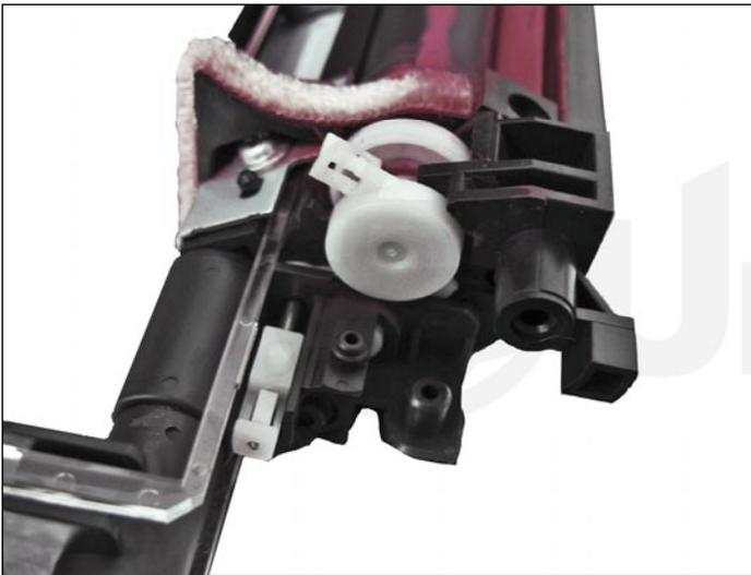
14. Remove the **capped** developer roller support bearing on the non-contact end cap side.
