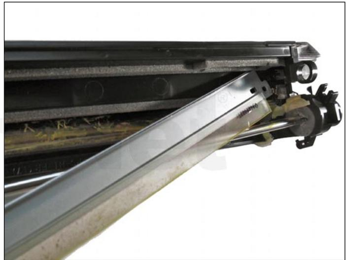
34. Remove the two wiper blade screws, and remove the wiper blade.
