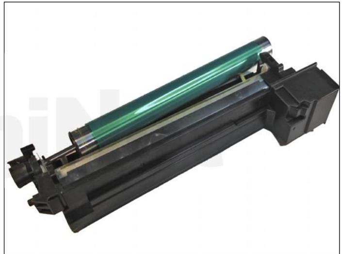
38. We are now ready to install the OPC drum. Before installing, make sure the drum gears are facing the correct position. Slide into place via the axle.
