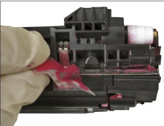
6. Remove the plastic cover off the top metal contact shown.
