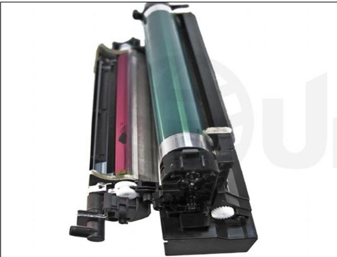
41. Assemble the two halves by first inserting the drive gear.
