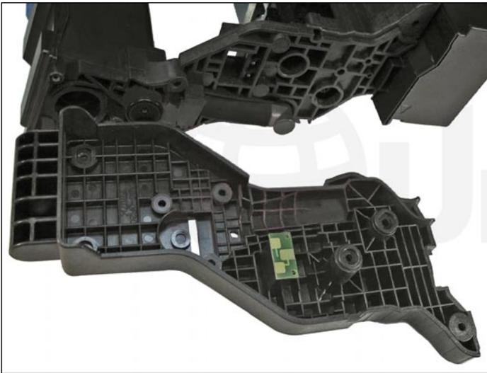
52. Install the **outer end cap** with the new chip installed.
