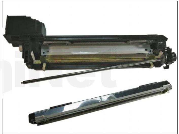
33. Remove the corona wire by sliding it in towards the opening on the gear train side (A), then pulling it out (B).
