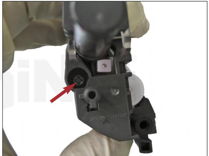
9. Remove the one screw from the **non-contact** end cap
