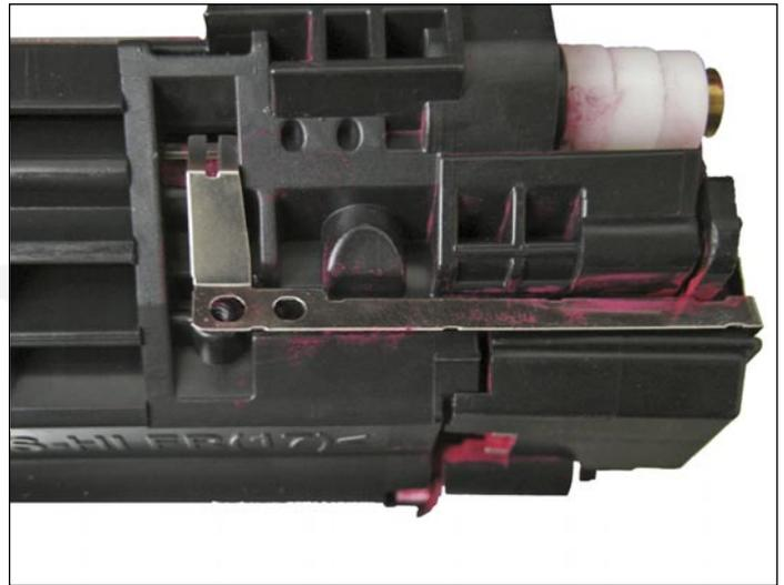
7. Remove the metal contact screws shown.
