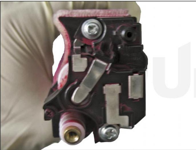
4. Remove the screws from the **contact** end cap.
