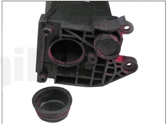
3. Locate the toner hopper fill plug, and remove it by prying it off, using a small flathead screwdriver.
