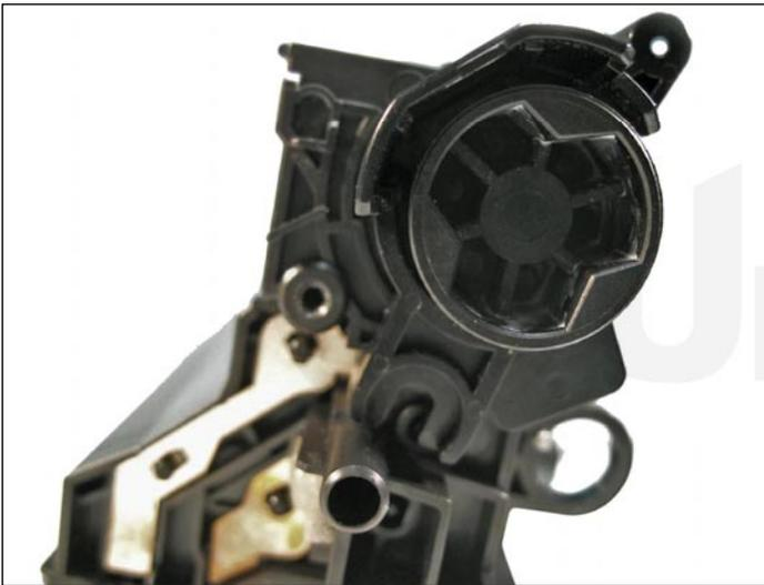
30. Final “unlocked” position of the drive gear support plate.
