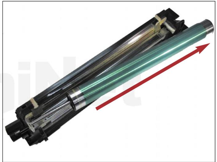
31. With the OPC drive gear support plate removed, this will allow movement for the drum axle and will simplify the removal of the OPC drum.
