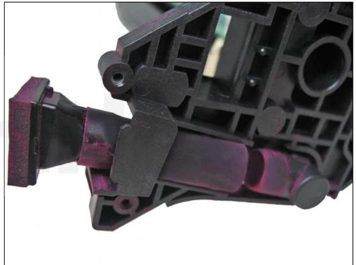
51. Install the transfer tube shown.
