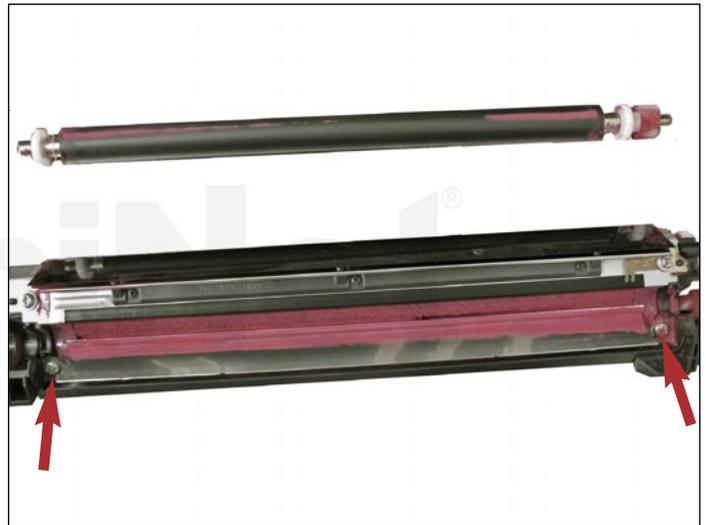
17. Remove the developer roller as shown.
